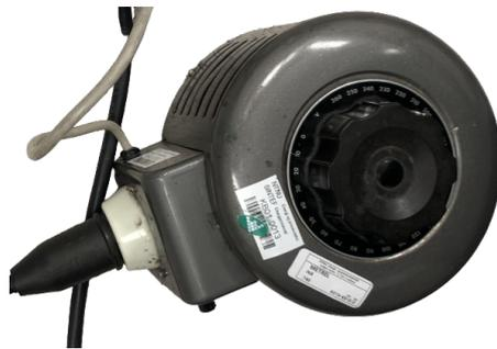
Figure 4.9: Voltage variable transformer used during the measurements to correct the output power of the thermal mannequin.
