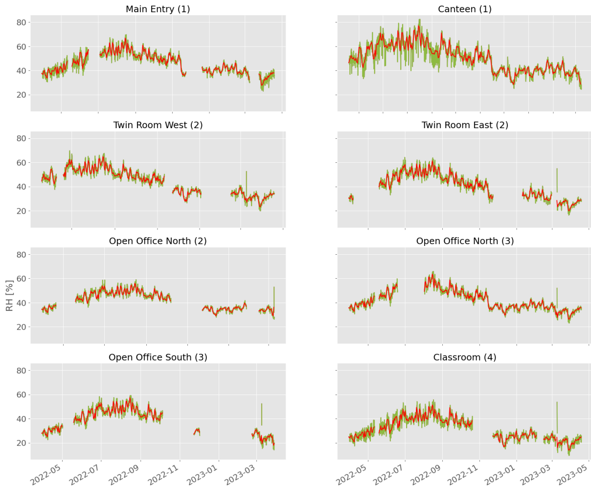
Figure 6.2.5: Hourly average (green) and 24-hour average (red) humidity levels in ZEB Laboratory.
