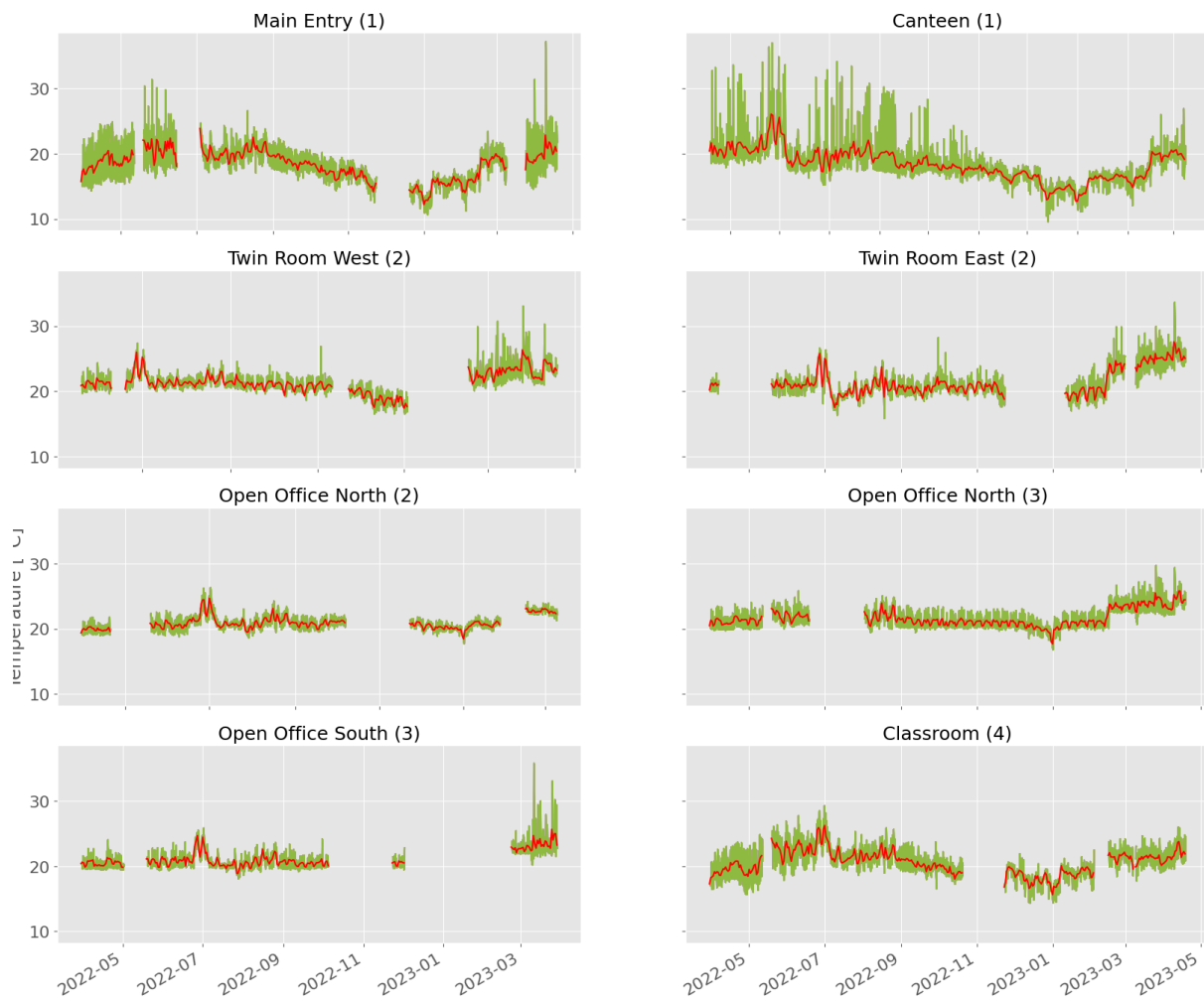
Figure 6.2.2: Hourly average (green) and 24-hour average (red) temperature levels in ZEB Laboratory.
