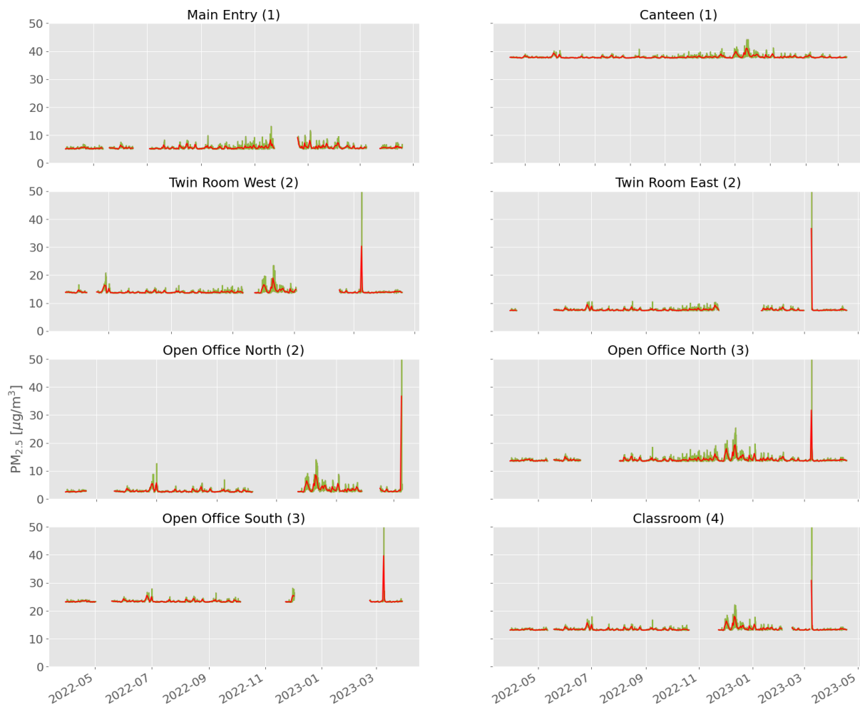
Figure 6.2.6: Hourly average (green) and 24-hour average (red) particulate matter ( 2.5 \mu ) levels in ZEB Laboratory.
