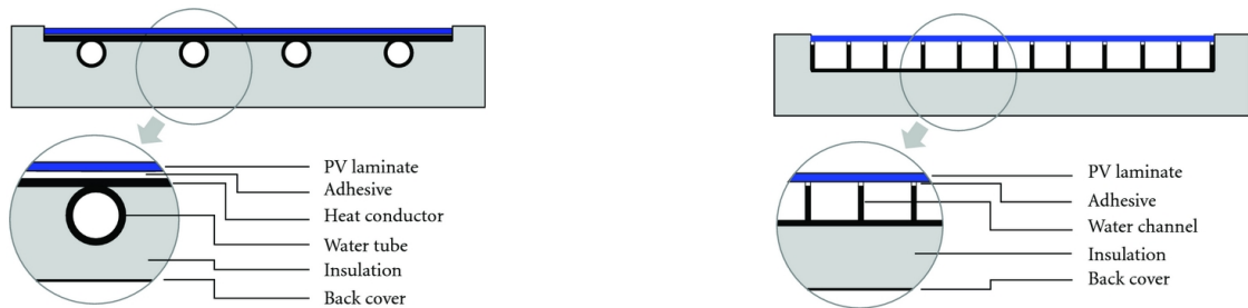
(a) Schematic of a sheet-and-tube PVT [20].
