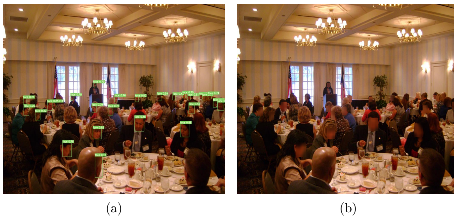
Figure 4.3.4: (a) Face detection using YOLOv7, (b) Face anonymization in meeting occasion.
