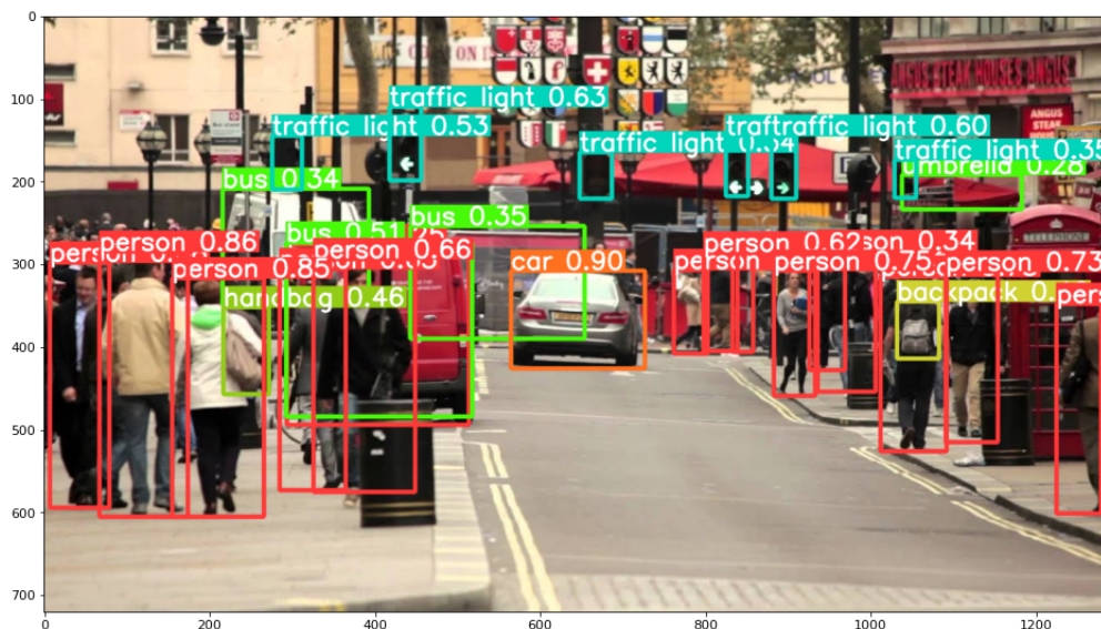
Figure 4.2.8: Real-Time Object Detection Inference in Python with YOLOv7 [51]
