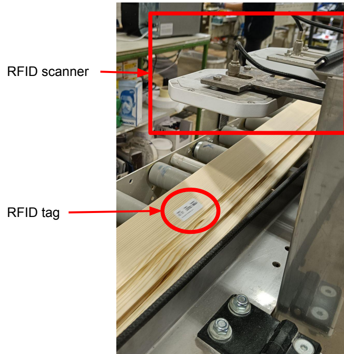
Figure 15: Photo of an RFID scanner and a component with RFID tag at Gilje's shop floor.
