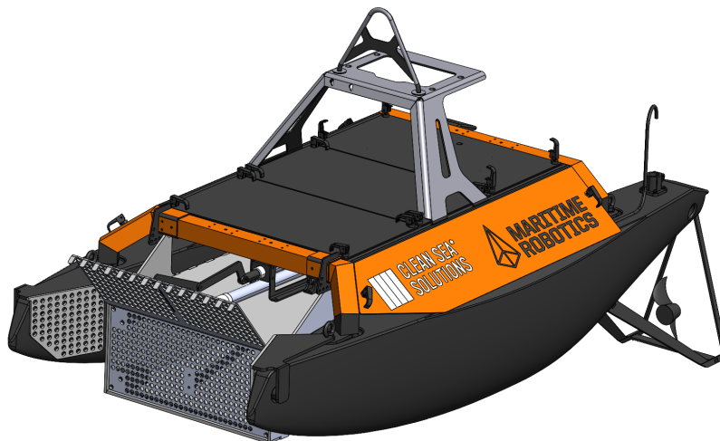
Figure 19: Aquadrone v1 with a early-phase collective system
