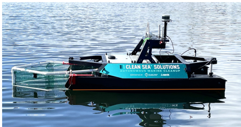
Figure 66: Visualized water-line along the hull proves a very stable position in the water(horizontal)
