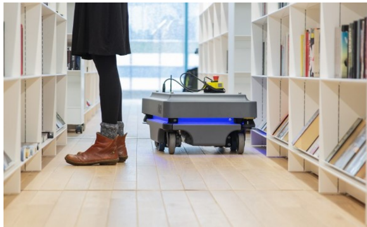
Figure 4: AGV employed at Oodi library, used to transport books between different floors.
