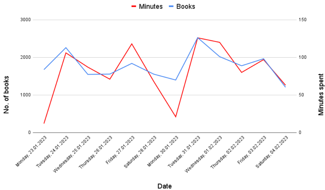
Figure 61: Books delivered and prepared for reservation plotted with minutes spent on material handling tasks categorized as material return.
