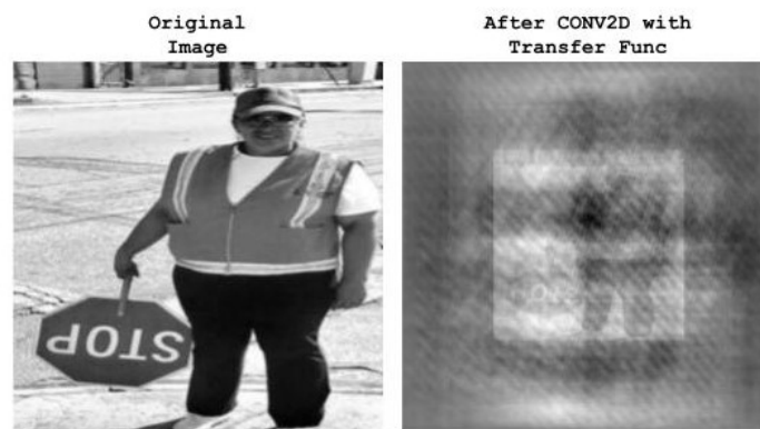
Figure 46: Example of using the transference function (PSF) on a different image to generate a flare artifact.
