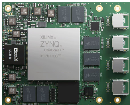
Figure 34: Zeus Zynq UltraScale [55]. Xilinx is a leading company in advanced programmable logic devices, particularly FPGAs
