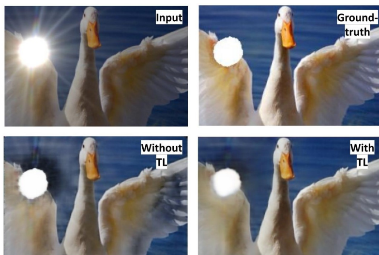
Figure 103: Inference using FlareNet model versions with and without transfer learning.
