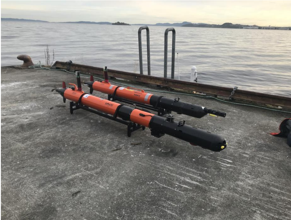
Figure 2.1: Two of AUR-Labs LAUV vehicles.
