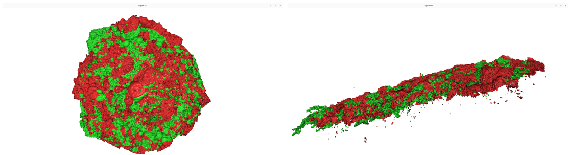
(c) Top view of aligned point clouds using RANSAC+ICP (d) Side view of aligned point clouds using RANSAC+ICP
