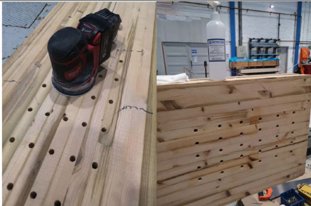
Before attaching the strain gauges to the weak end, the surface was sanded and cleaned
