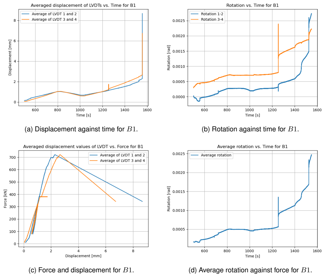
Figure 45: Data from LVDTs on B1 .
