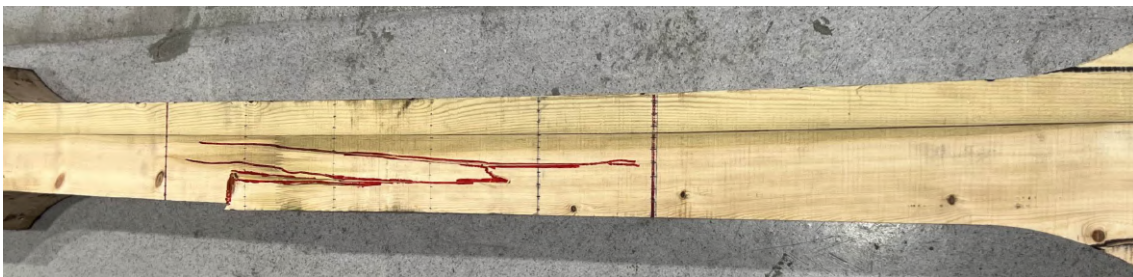
Figure 58: Failure in tension zone with secondary shear failure.
