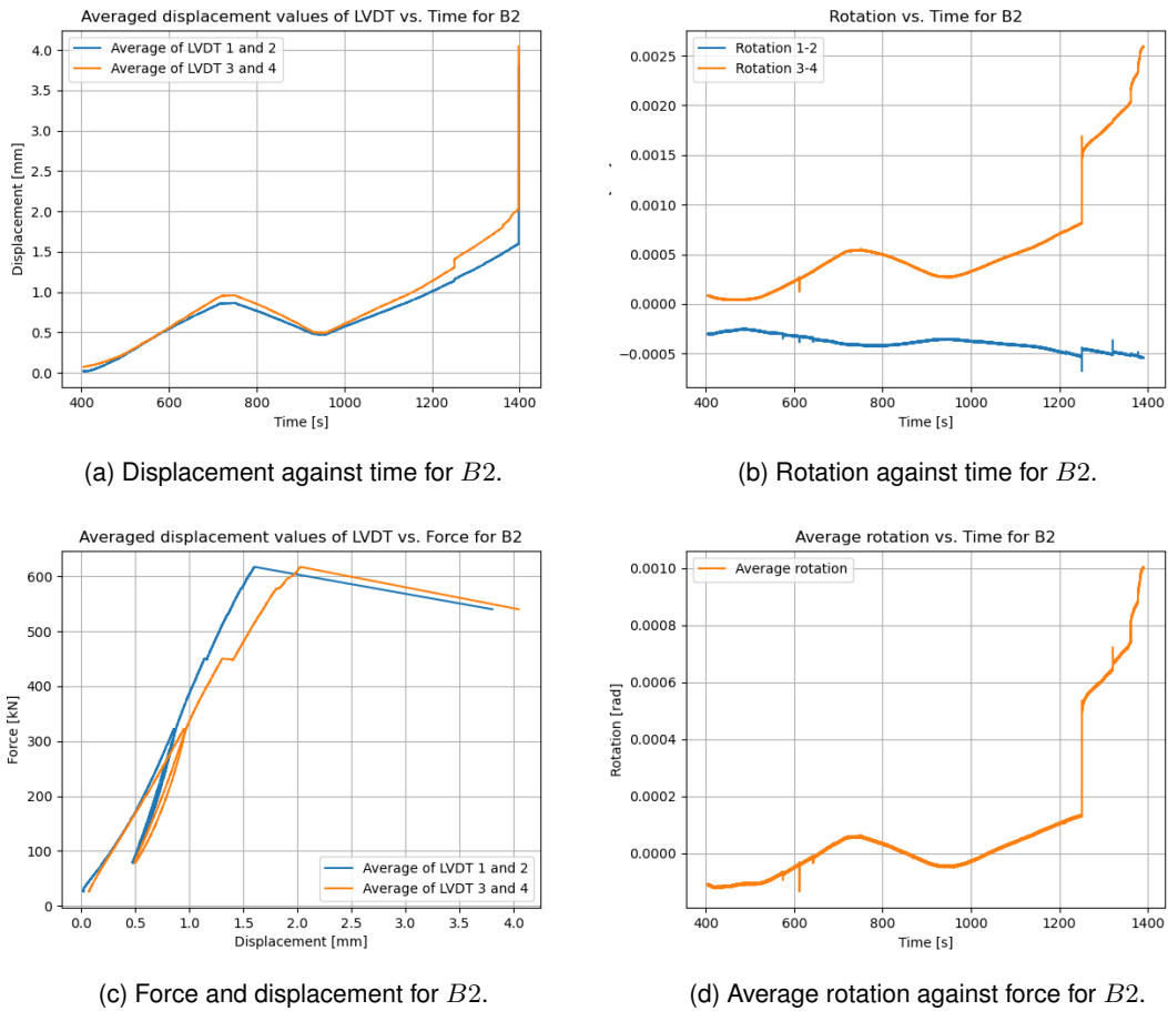
Figure 46: Data from LVDTs on B2.
