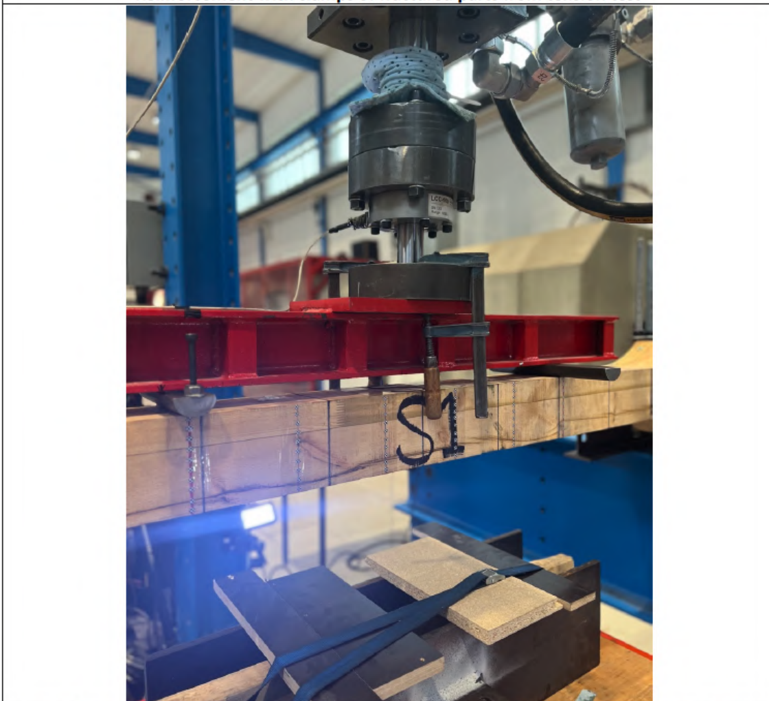
Horizontal beam secured with clamps and lasers protected from falling fracture parts
