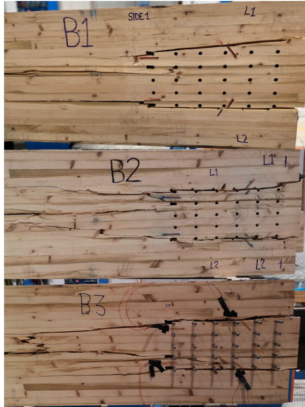
Figure 43: Visualization of block failure surfaces.
