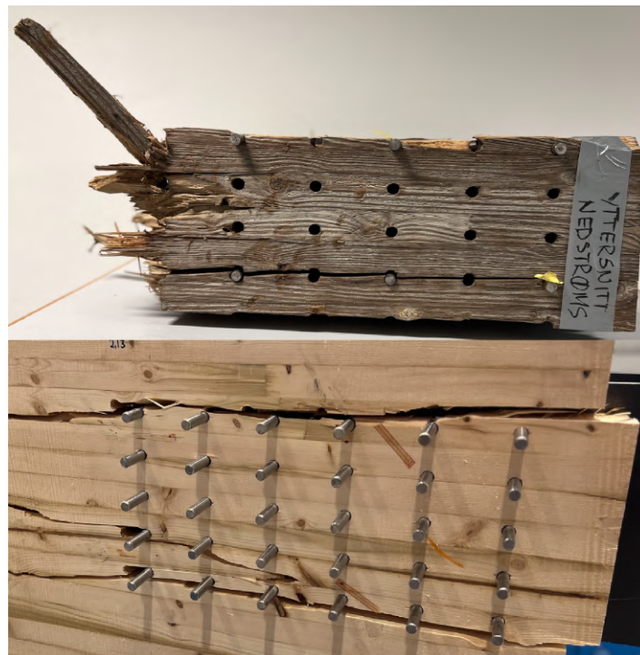
Figure 1: Decisive block failure from Tretten bridge and experiments.
