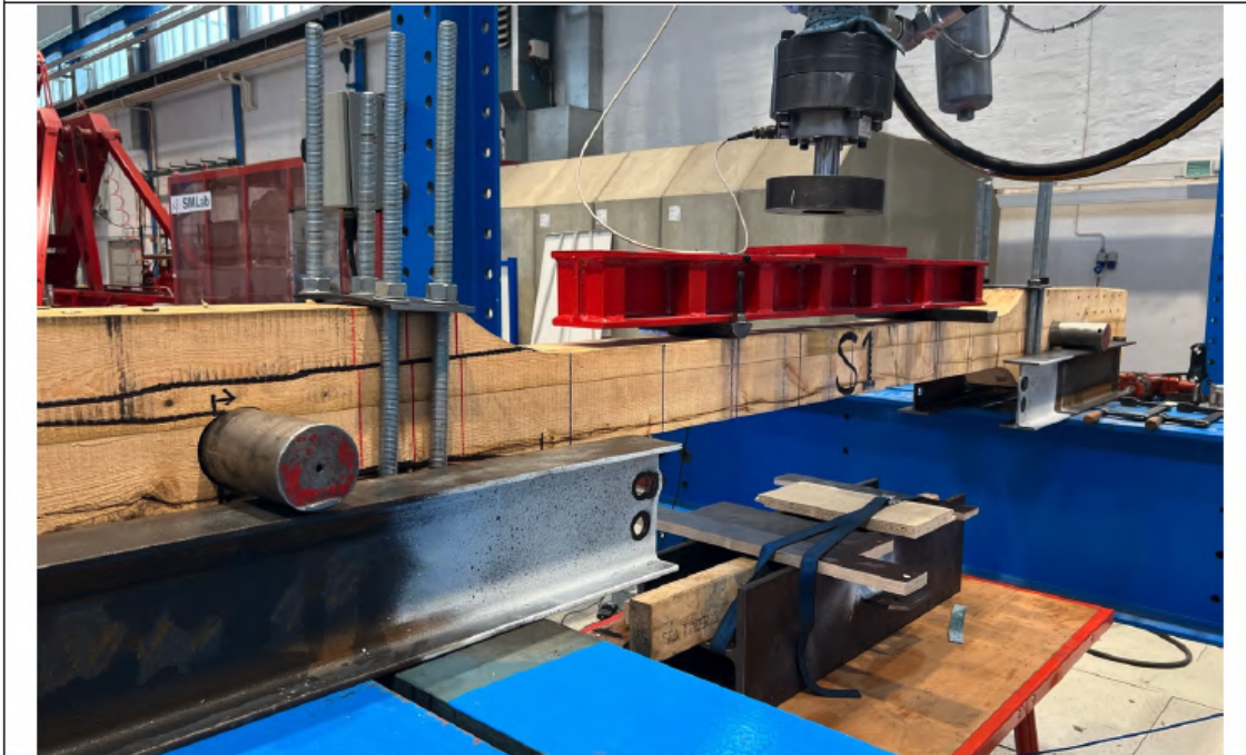
Reinforcement with clamps of fractured parts from tension test
