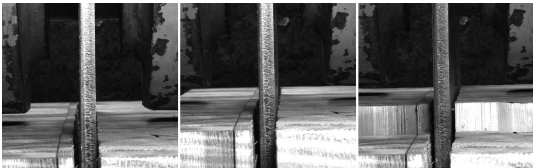
Figure 34: Camera pictures at start, before and after block failure of B1 .
