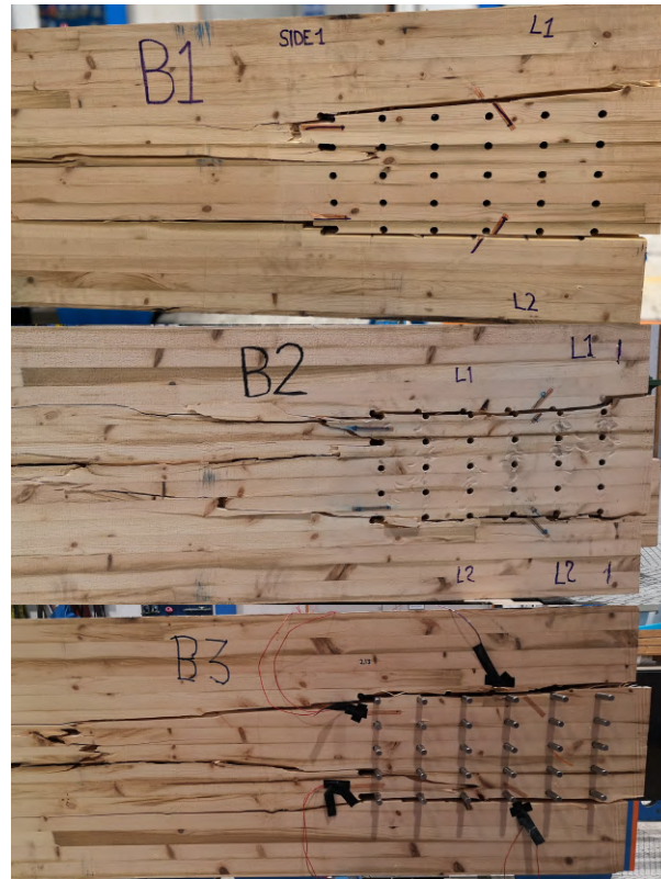
Figure 30: Visualization of block failure surfaces.
