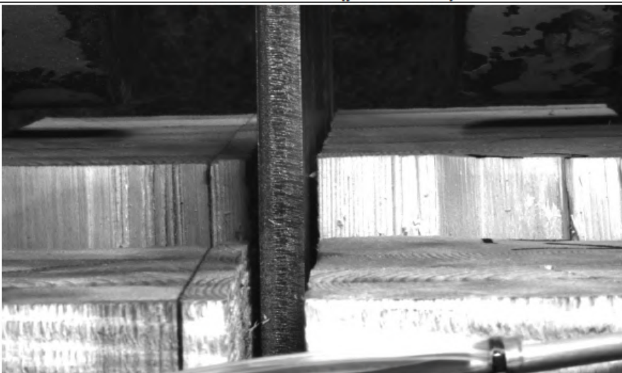
Block failure (picture 1549)
