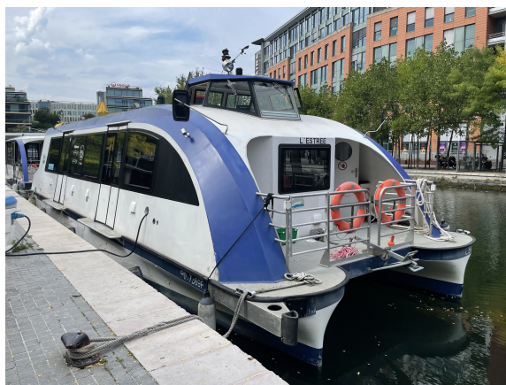
Figure 1.5: Paris river shuttle that operates in the channels of Paris. These shuttles are underactuated and electric. Courtesy of Øyvind Smogeli.
