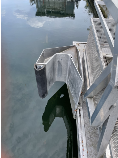
Figure 1.7: A docking receiver that is used to simplify docking for underactuated vessels. This receiver is installed in the docks in Paris to mate with docking hitches equipped on the ferries. The dock in the simulation environment will be modeled with such a docking receiver. Courtesy of Øyvind Smogeli.
