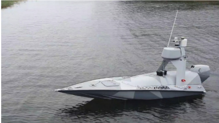
Figure 2.1: The Piraya, an experimental USV platform developed by Saab Kockums (Saab, 2022). The vessel is underactuated with only an outboard engine at the back. Picture is from (Kockum, 2022).
