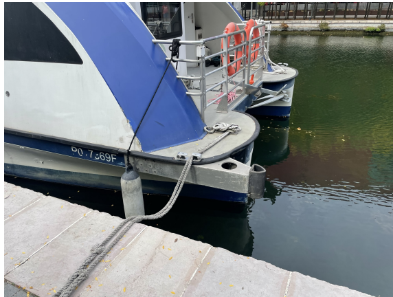
Figure 1.6: A docking hitch that is used to simplify docking for underactuated vessels. The passenger ferries in Paris are installed with such hitch as pictured here, and the Otter model used in this thesis is supplied with one as well. Courtesy of Øyvind Smogeli.
