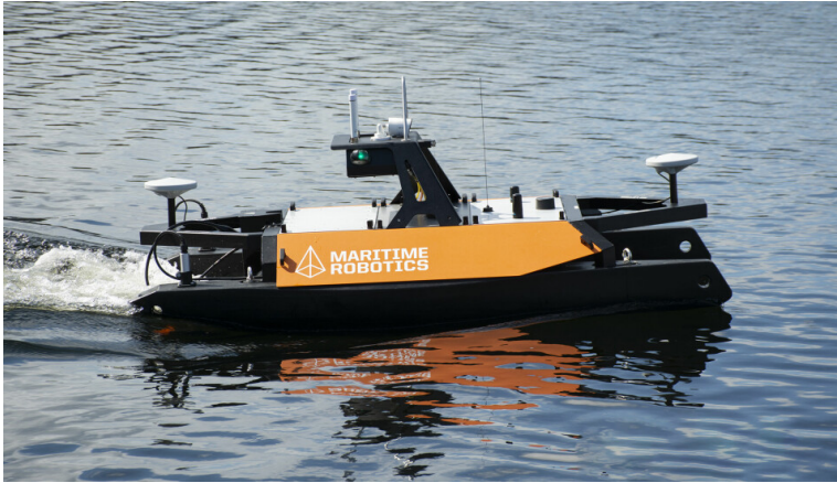
Figure 3.1: The USV Otter, an unmanned surface vessel platform developed by Maritime Robotics (Robotics, 2022).
