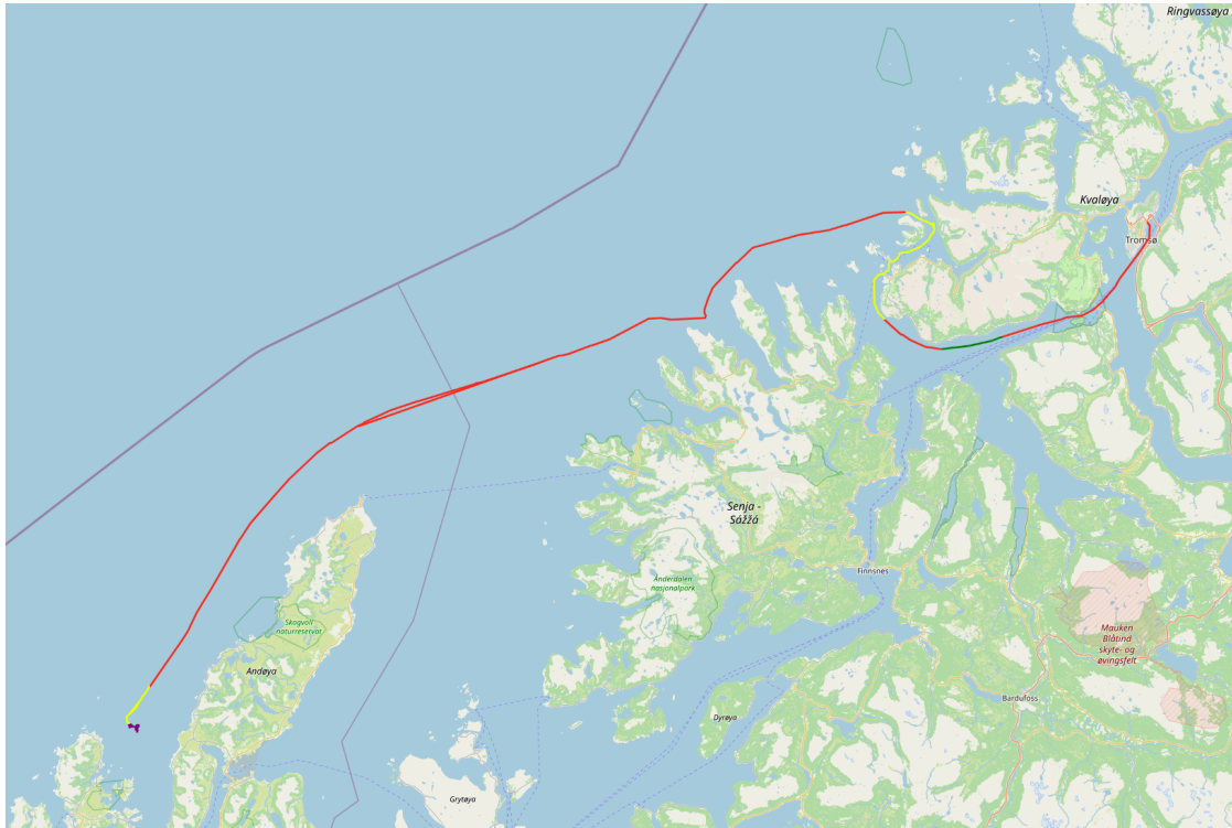
Figure 4.9: CNN and k -means predictions. Yellow trajectories depict times when the vessel is searching for fish, while red and green trajectories depict times when the vessel is steaming. Purple trajectories depict times when the vessel is fishing.
