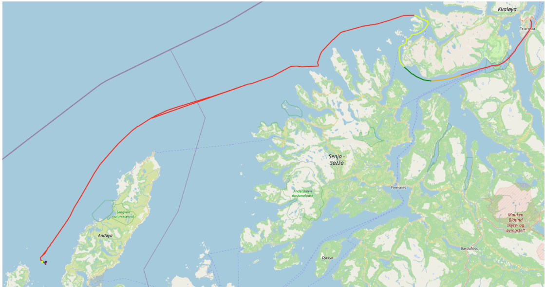
Figure 4.25: k -means predictions with 0 as padding value. Yellow trajectories depict times when the vessel is searching for fish, while red/green trajectories depict times when the vessel is steaming. Orange trajectories depict sections where the data quality was below the resolution demand. Purple trajectories depict times when the vessel is fishing.
