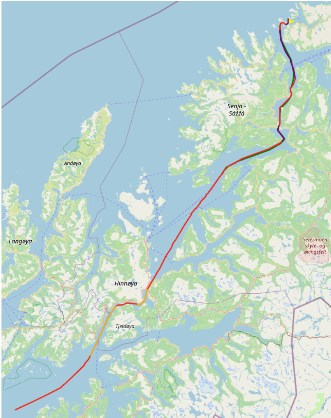
Figure 4.27: k -means predictions with 0 as padding value. Yellow trajectories depict times when the vessel is searching for fish, while red/green trajectories depict times when the vessel is steaming. Orange trajectories depict sections where the data quality was below the resolution demand. Purple trajectories depict times when the vessel is fishing.
