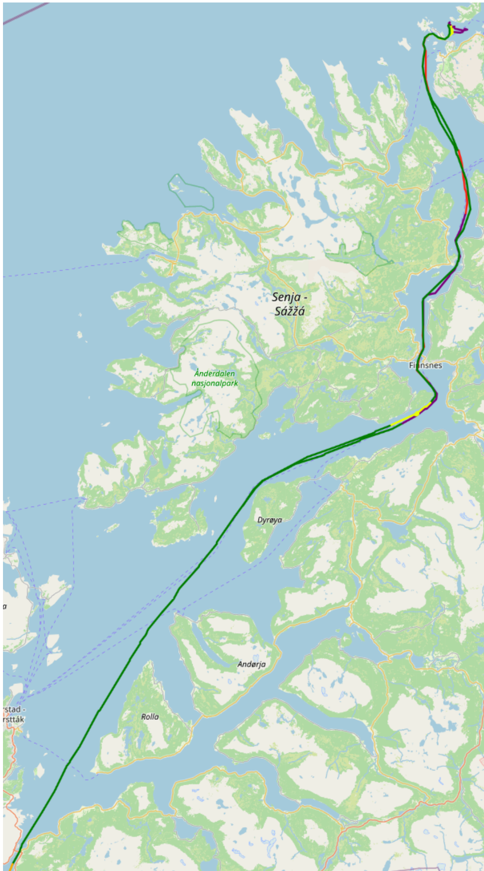
Figure 4.35: k -means predictions for feature-based dataset. Yellow/purple trajectories depict times when the vessel is searching/fishing; this is unclear. Red/green trajectories depict times when the vessel is steaming. Orange trajectories depict times when the data quality was below the resolution demand.
