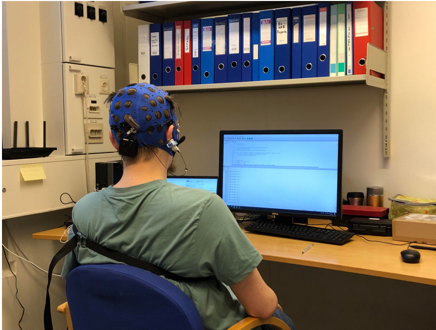
Figure 3.5: Set up example. Subject is wearing the EEG cap, and the fastening of the reference electrode on the right earlobe is visible. The PCG is placed under the t-shirt on Erb's point and fastened using the black buckle strap.
