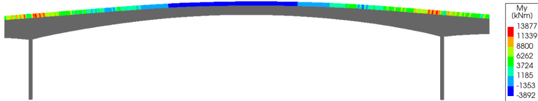
Figure 57: Distribution of bending moments, M_{y,Ed} , along the central part when the bridge is subjected to load case ULS a.
