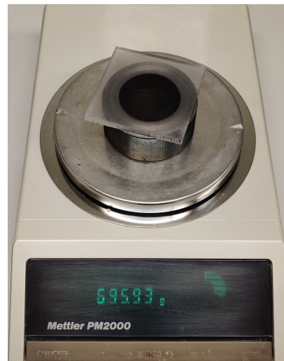
(b) Weight of cylinder filled with water
