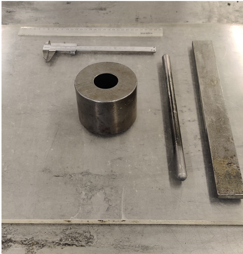
Figure 2.8: Equipment for mini-slump test: mini-slump cone, plexiglass, compacting rod, steel bar, rulers
