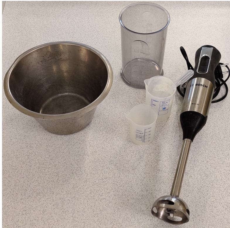
Figure 2.4: Equipment for mixing filler-modified cement paste: metal bowl for dry particles, beakers for water and SP, with pipettes and a the hand-blender
