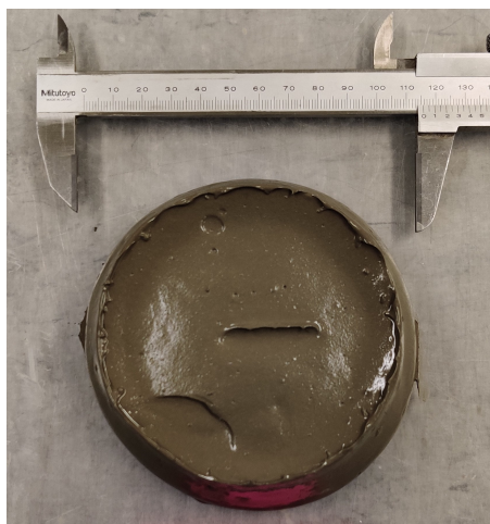
(a) Measuring mini-slump flow value for G2T815W4
