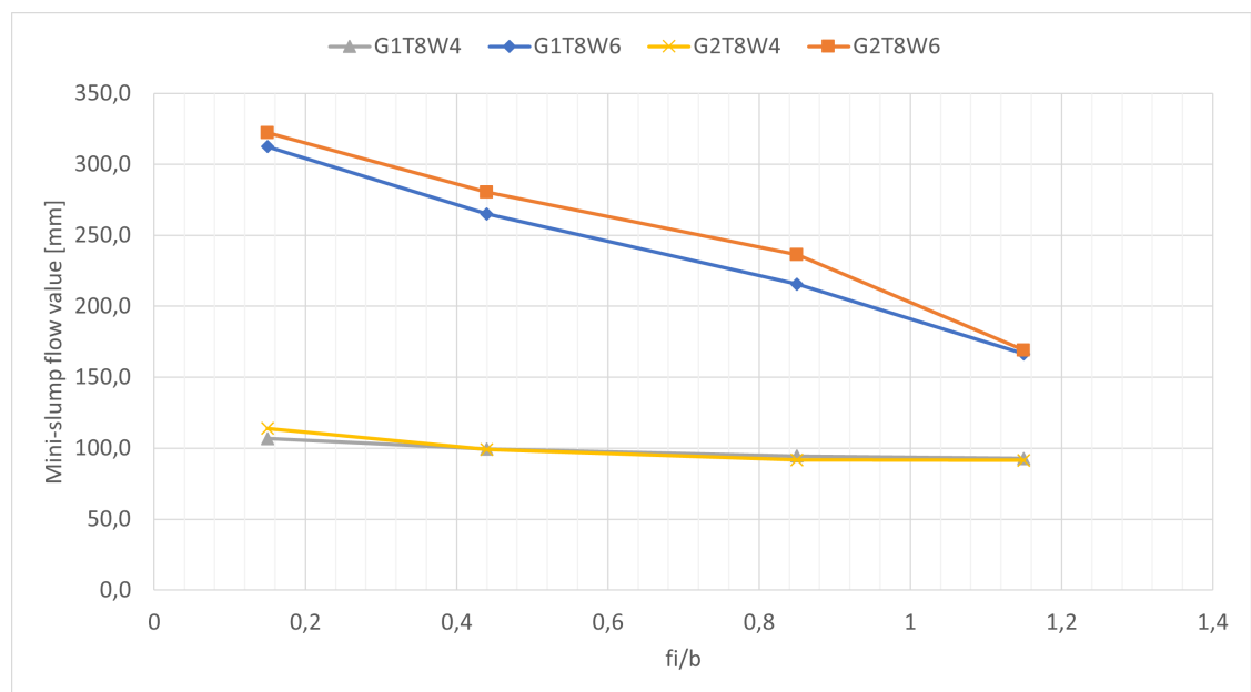
Figure 3.4: Mini-slump flow value of mixes using filler T8 plotted against f_i/b
