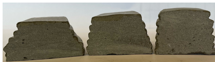
(a) Hardened printability test specimens that has been cut, left to right: G3T515W4, G3T544W4, G3T585W4
