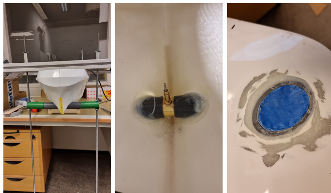
Figure 4.2.1: Installation process for bow thruster
