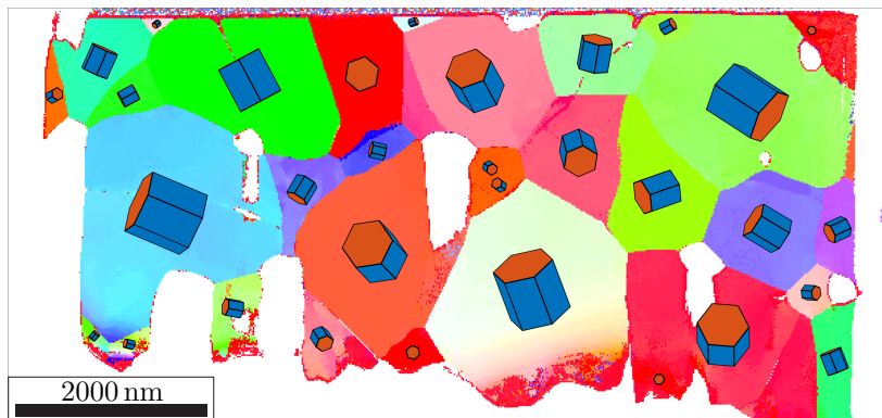
Figure 4.7: Crystallographic orientation of grains in the sample with unit cells plotted on top of each grain.
