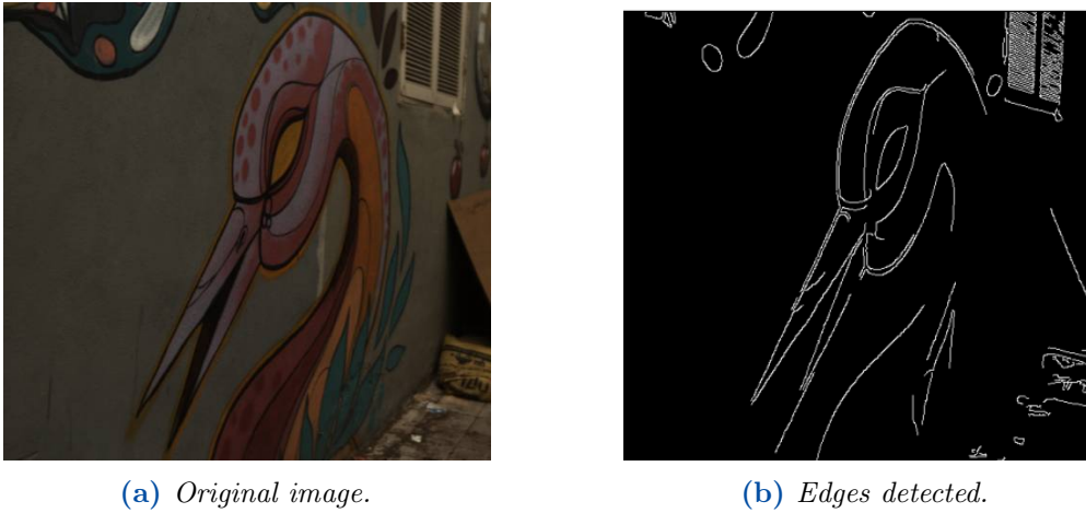
Figure 3.7: Detected edges using Canny edge filter to isolate them and generate their saliency maps.
