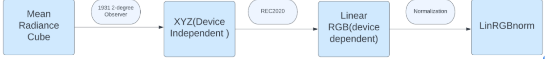
Figure 4.16: The figure illustrates the proposed workflow for converting hyperspectral HDR radiance cube into HDR three-channel RGB image which is finally stored in 32-bit float using .hdr format which is basically a mapping of the visible spectrum of HDR hyperspectral radiance cube to the XYZ color space and from there to the Rec. 2020 color space.
