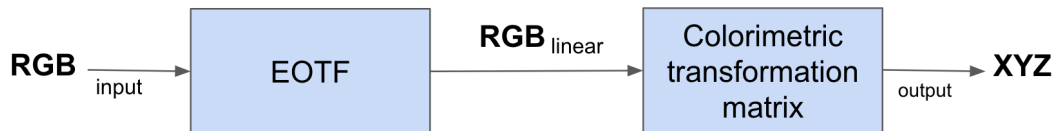
Figure 6.7: The display model involves the display's Electro-Optical Transfer function (EOTF) and the colorimetric transformation matrix.
