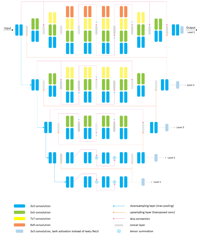
Figure 2.5: Architecture Details of PyNet Model. Image from Ignatov et al. (2020b)
