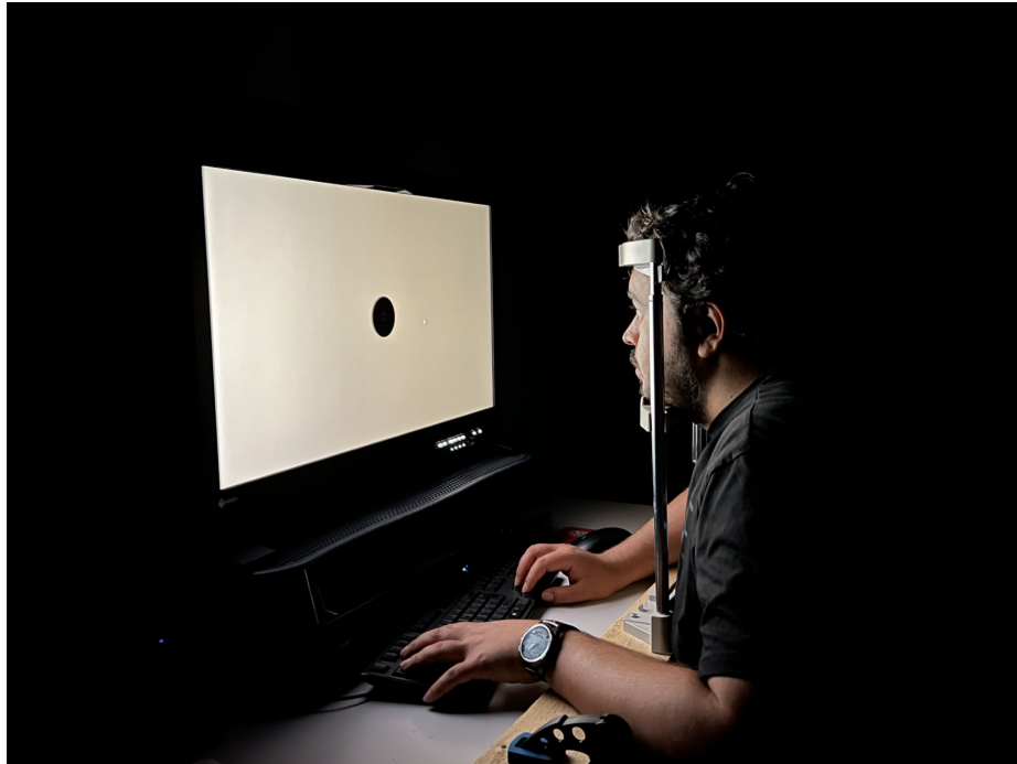
Figure 3.10: Experiment setup with display, chin rest and observer.
