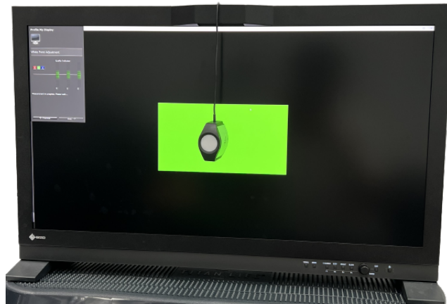
Figure 3.6: Calibration with x-rite i1 display pro of EIZO Prominence CG3146 display.
