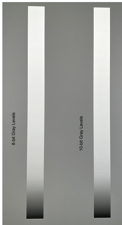
((a)) High Dynamic Range image generated with 8-bit gray level and 10-bit gray level gradients, displayed on HDR Eizo screen using psychtoolbox in Matlab. The presented levels illustrate the degree of transition smoothing in both 8-bit and 10-bit systems. It is expected that the 10-bit system would exhibit a higher level of smoothness compared to the 8-bit system when viewed on a HDR screen.
