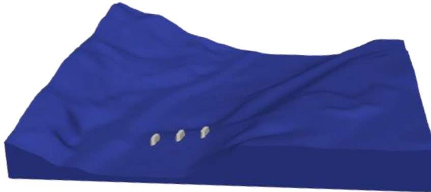
Figure 12: The STL file of the terrain is shown in blue and the STL file of the piers is in white.
