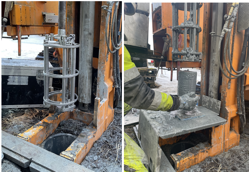
(a) Mini block sampler before sampling. (b) Mini block sample immediately after sampling.
