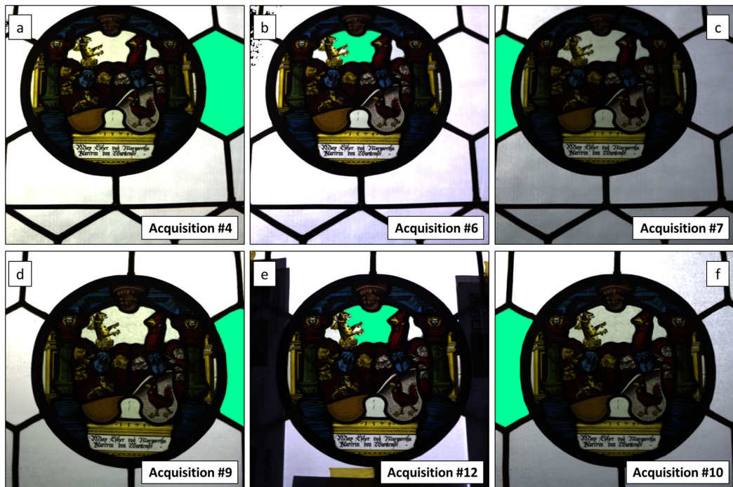
Fig. 8 Pictures showing the areas chosen as transmittance reference (in green) for the acquisitions #4 to #12 of the case study AG-1177. The differences between the pictures in the first row and the ones in the second row are due to the inclination of the camera during the recording of the first set of images. Acquisitions #4 and #9 (a, d), #6 and #12 (b, e) and #7 and #10 (c, f) were processed using the same glass pane. Some paper sheets were also placed on the sides of the panel during acquisition #12 to decrease the contrast between the dark colored glass and the transparent ones
