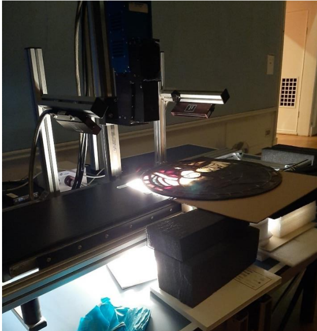
Figure 4.4: Configuration of the setup during the acquisition of Vigeland's stained-glass panels. An extended support was used to handle large-sized objects.
