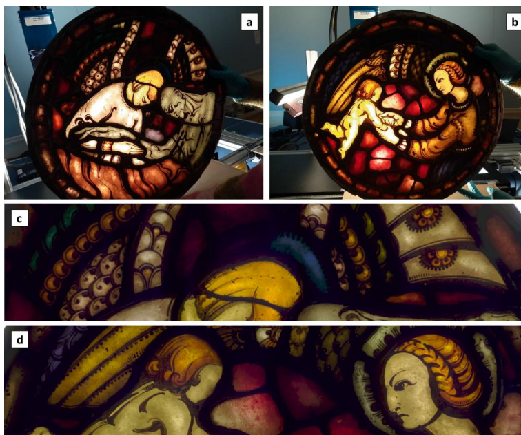
Figure 4.3: a, b) the two Vigeland's stained-glass panels analyzed at the old building of the National Museum of Oslo. Notice the darkness of the glass pieces and the presence of a thick patina applied over all the glass pieces. c, d) RGB images rendered from the datacube through color matching function and a standard illuminant (D65). Note that the brightness has been slightly increased to improve the visualization of darker colors (e.g., green, blue, and purple).
