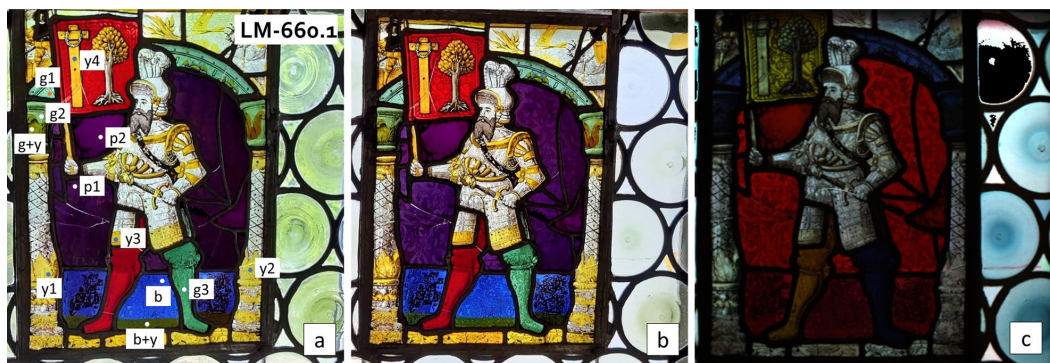
Fig. 20 a Close-up picture of case-study LM-660.1, showing the points selected for the spectra comparison. b Close-up picture of case-study LM-660.1, after the application of the diffusing sheet. c False-color image obtained from acquisition #6
