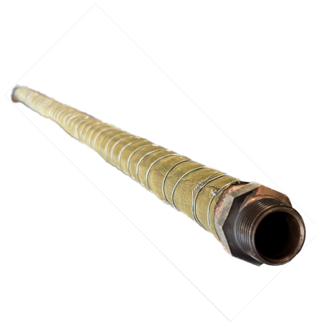
Figure 8.2: Inner pipe of collector
