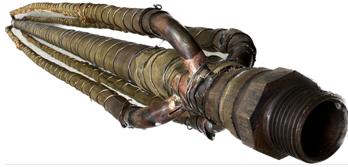
Figure 8.13: Methanol dispenser inside the collector. Extended capacity with four extra pipes to increase heat transfer and methanol dispersion.
