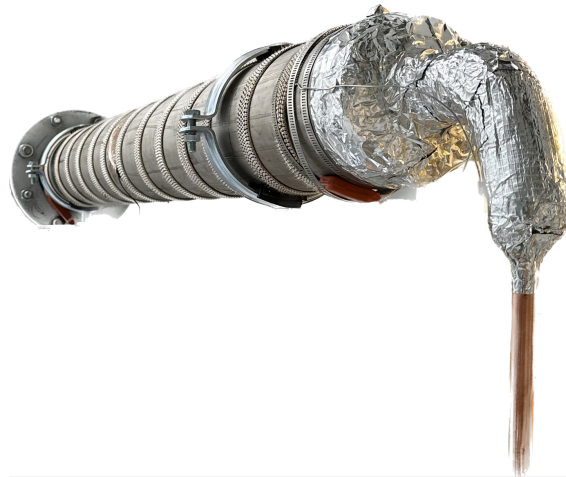
Figure 9.6: Added insulation around the collector outlet for increased recording accuracy, and reduced heat loss
