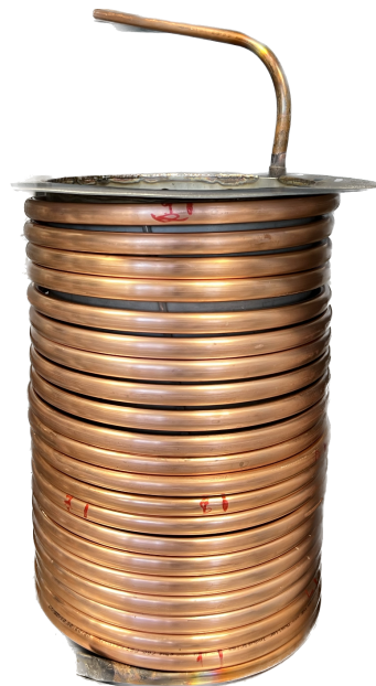
Figure 8.5: Evaporator coil wrapped around the refrigerated chamber. The coil on top is the inlet from the condenser.
