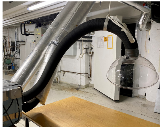
Figure 6.2: Odour supply hood.
