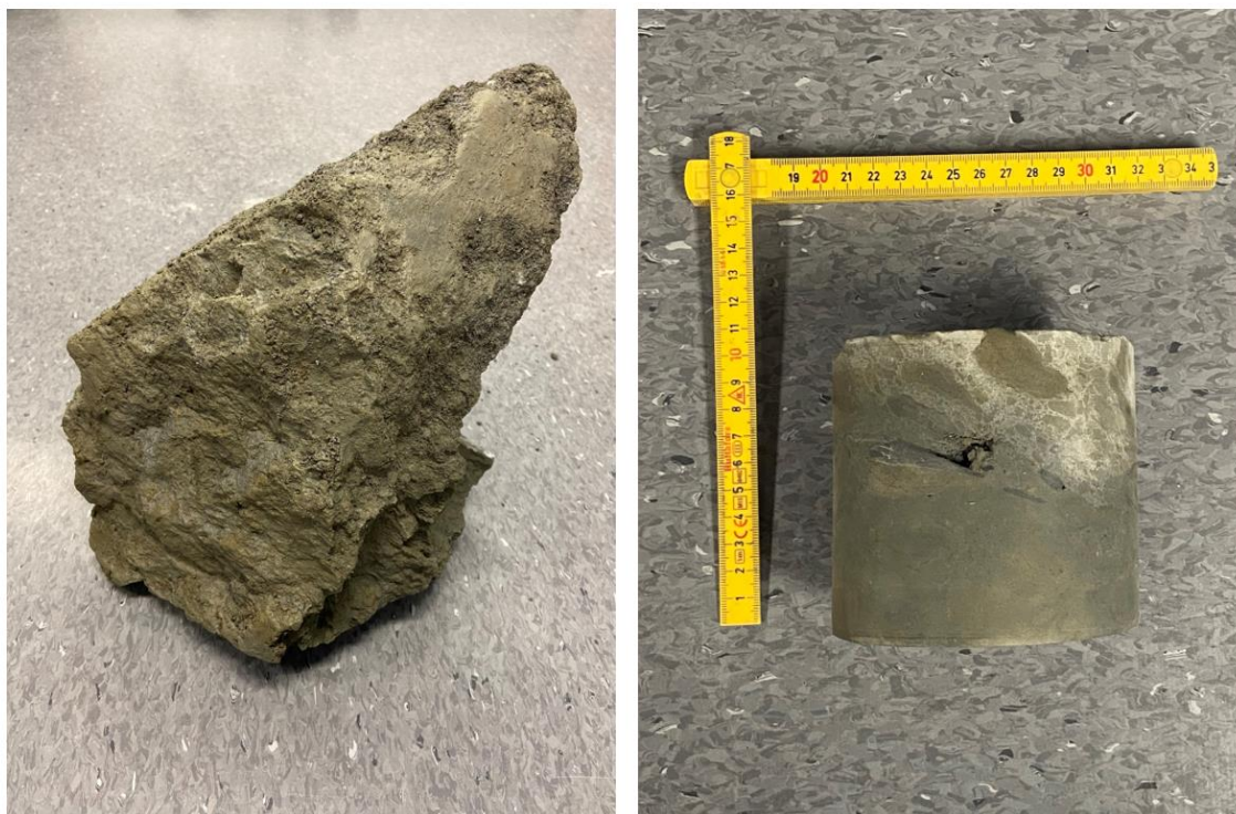
Figure 27: MDM sample before and after trimming.
