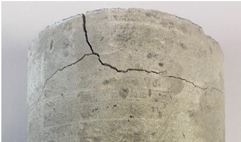
Figure 60: Visible surface cracking in the upper section of the WDM.Hjorthagen.3 sample.
