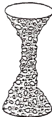
Figure 17: Typical concrete cylinder sample fracture pattern (Jacobsen et al., 2022).
