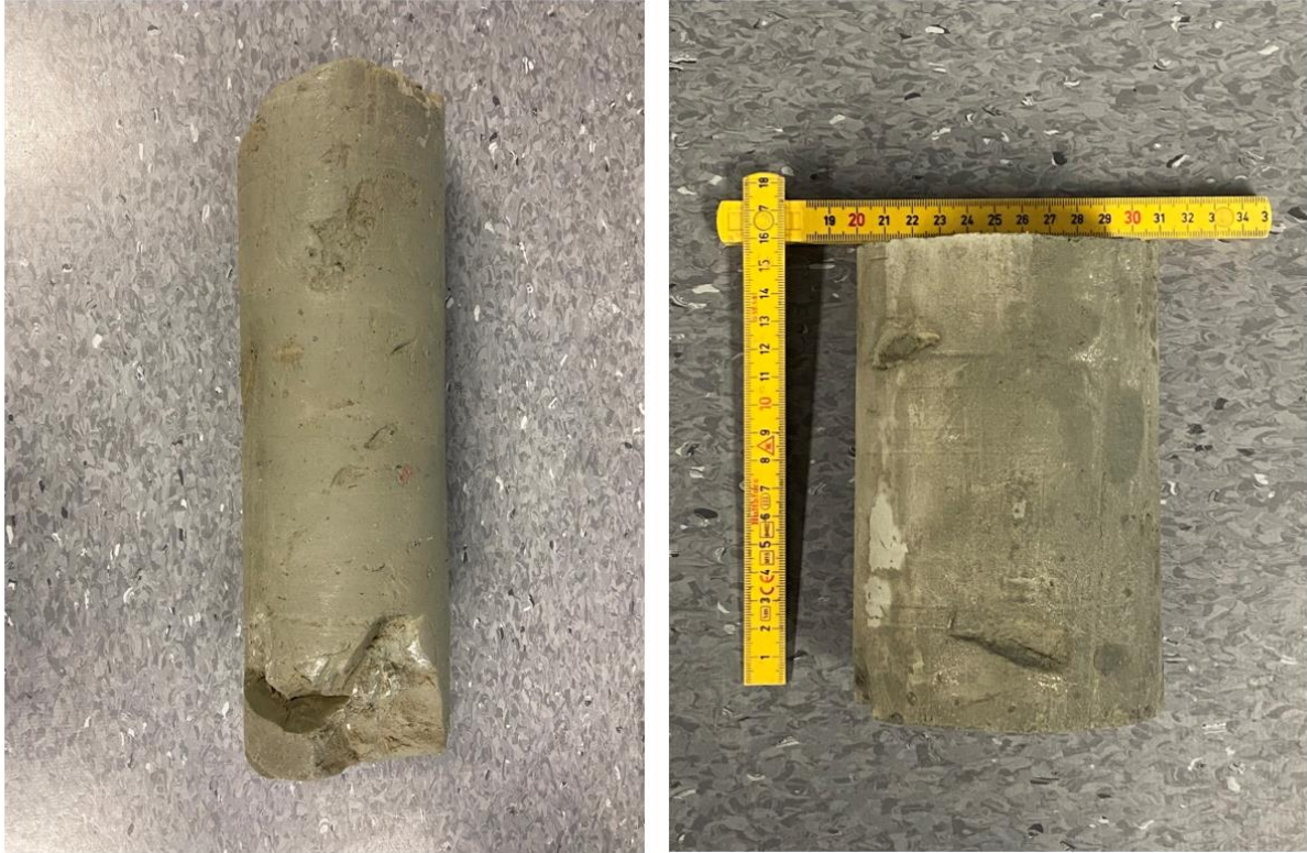
Figure 28: WDM sample before and after trimming.
