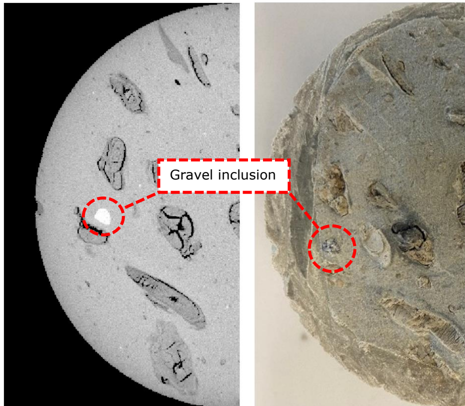
Figure 66: 2D \mu CT image (left) vs physical sample image (right) showing a small piece of gravel as an inclusion in the WDM.Östrand.2 sample at slice 1072.
