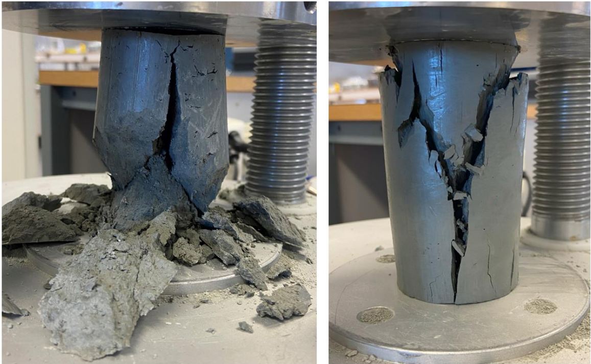
Figure 70: Combination of a cone and longitudinal fracture pattern.
