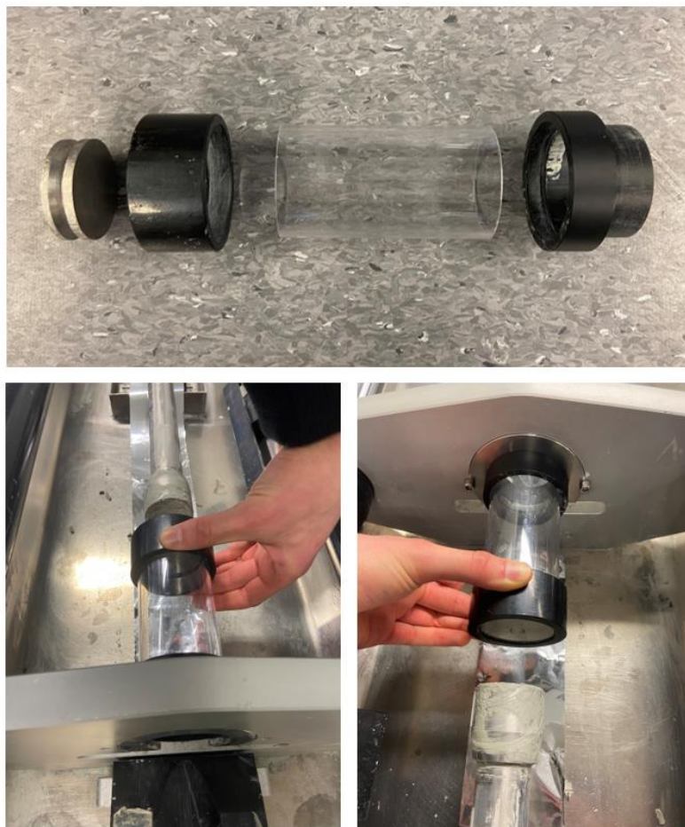
Figure 37: Hydraulic extrusion equipment for cylinder samples.
