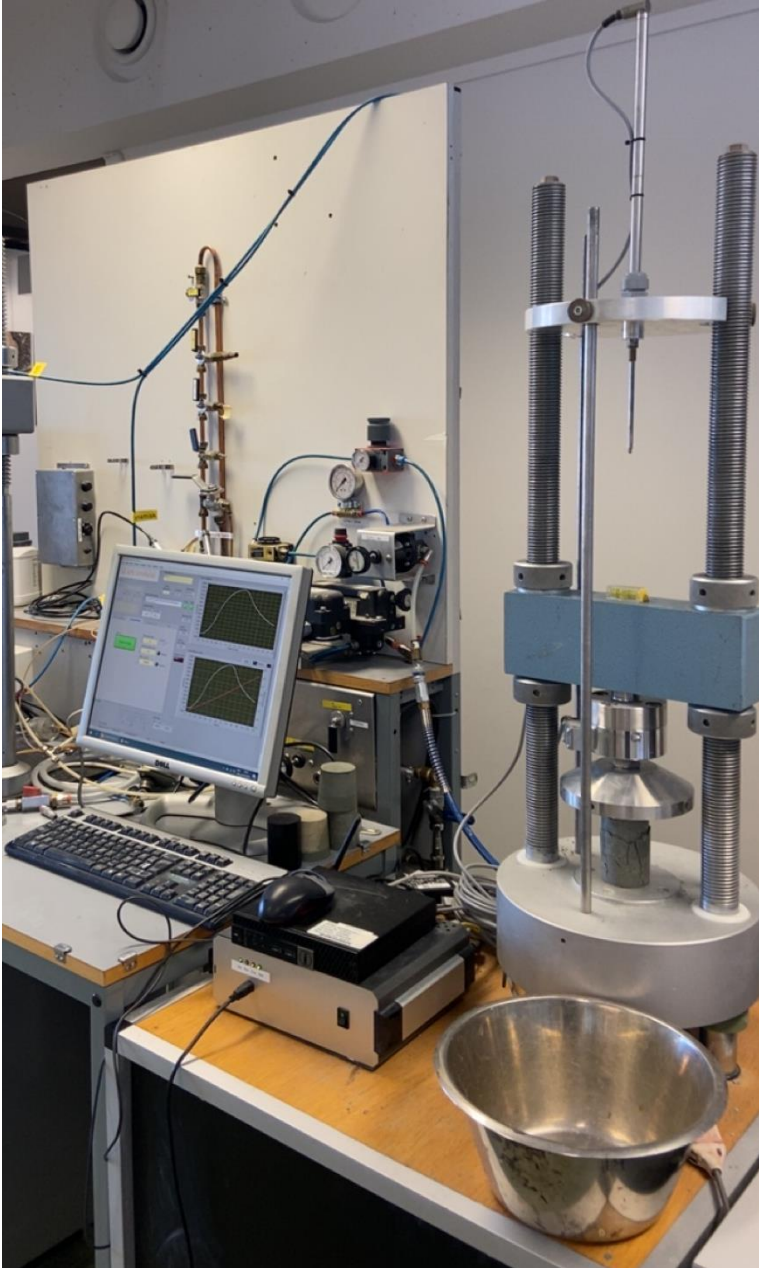
Figure 41: Unconfined compression test equipment setup.
