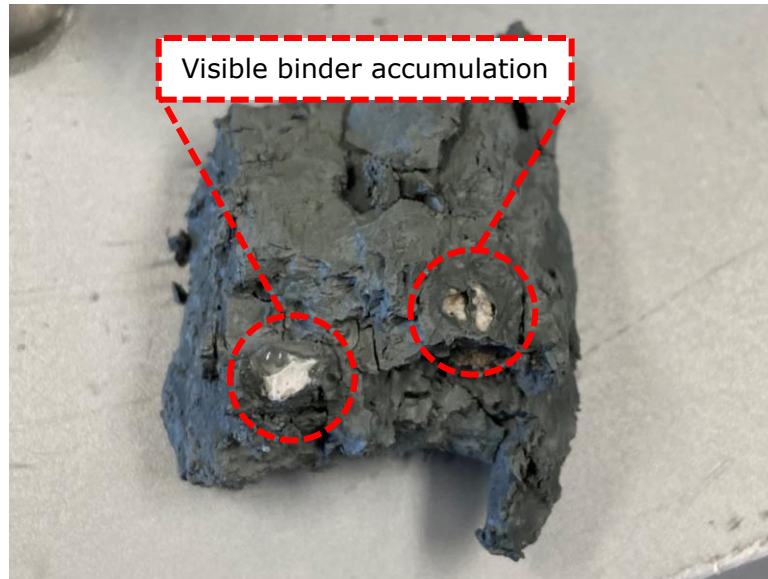
Figure 69: Binder accumulation in a dry mixed sample.
