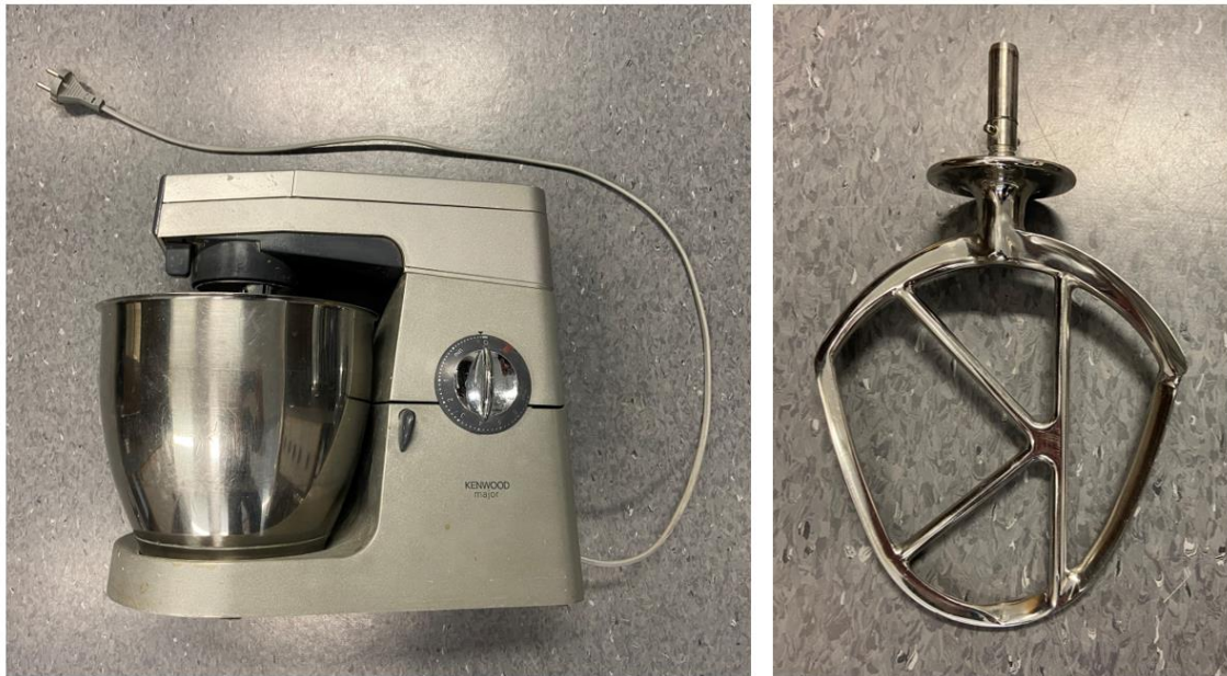
Figure 34: Kitchen stand mixer (left) and k-type mixing tool (right) used to prepare batches of stabilized soil.
