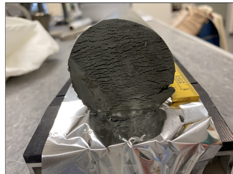
(b) Cracks while cutting near bottom sample 4
