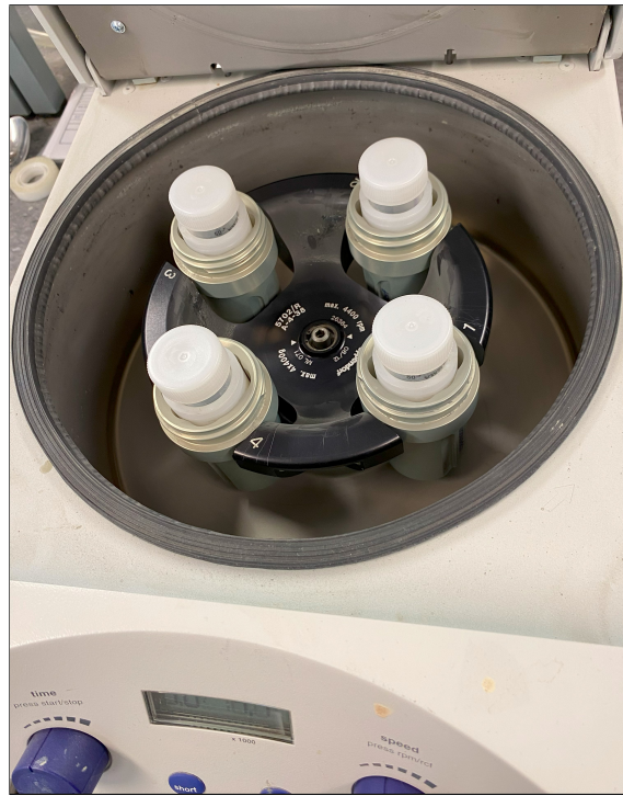
Figure 1: Pore water extraction using centrifugation device
