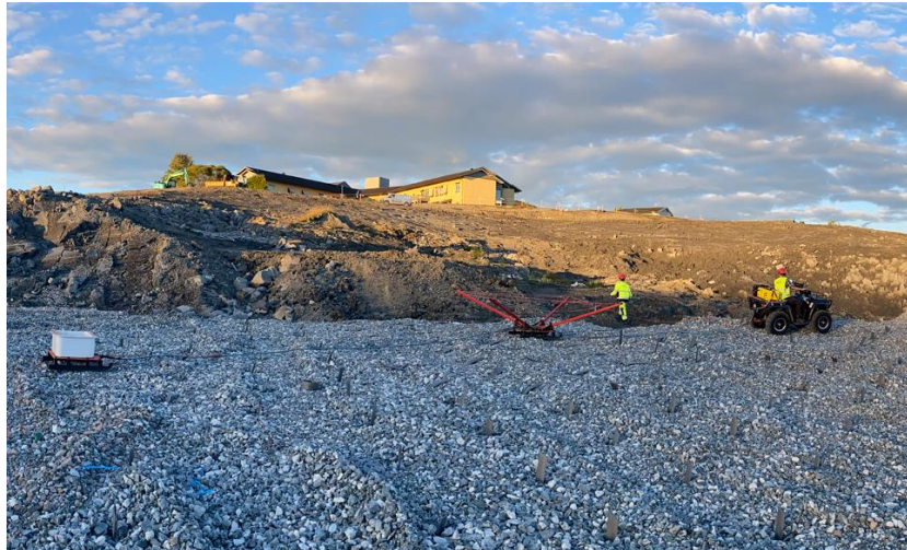
Figure 23. tTEM survey in the landslide area. Photocredit: Christos Boufidis and Søren Bjørn
