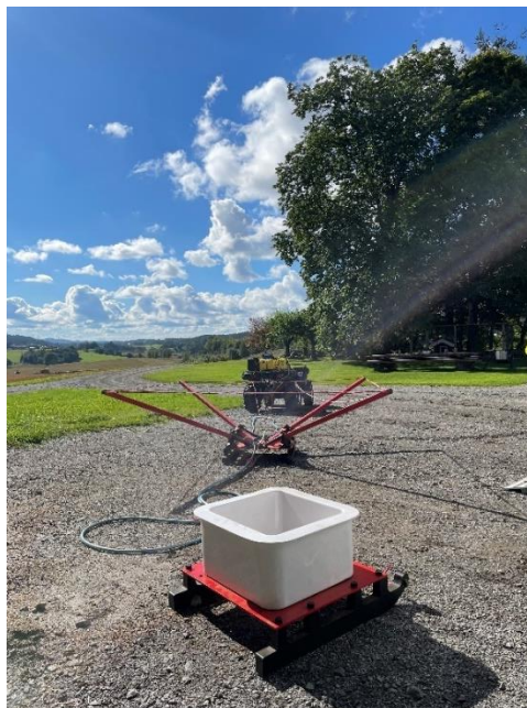
Figure 22. tTEM-equipment used in Gjerdrum. Photocredit: Christos Boufidis and Søren Bjørn
