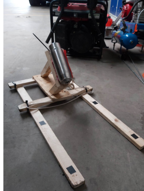
(a) Wooden mount with the camera at an angle to the surface.
