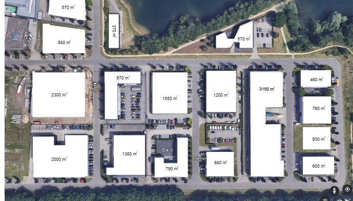
Figure 4.18: Data on roof catchment/area were mapped and linked to the nearest manhole to create relevant illicit inflow scenarios in the model.
