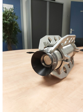
(b) 3D printed cone used for reducing light reflections.
