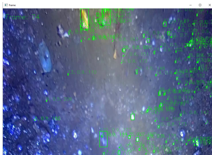
Figure 3.6: Screenshot from the particle identification procedure in the PTV algorithm in footage in ultraviolet/visible light. Data on the particles are displayed with the particle outline. Current frame particles are compared with particles detected in previous frames to obtain track their trajectory.
