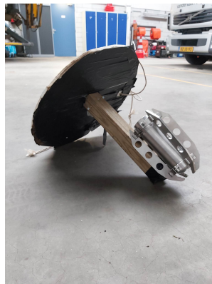
(a) Wooden cover/mount giving a birds-eye-view of the manhole.
