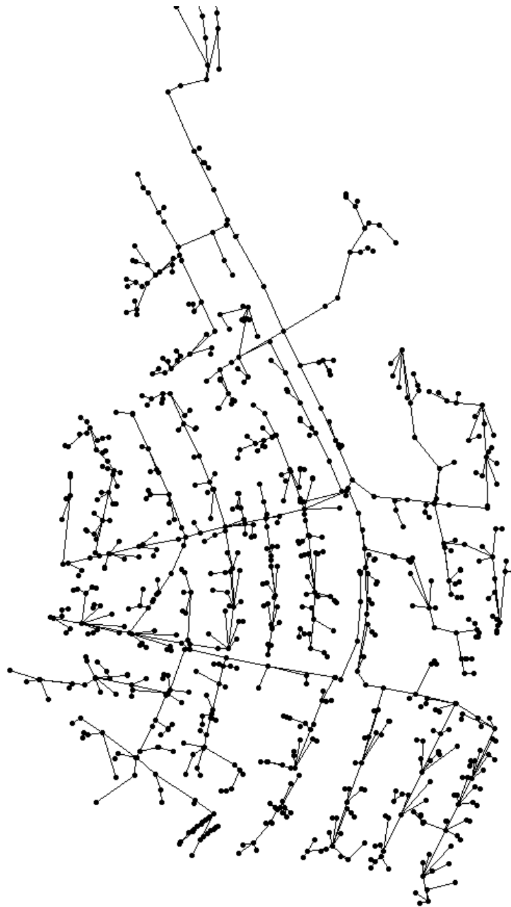
Figure 5.9: Holtandalen EPA-SWMM model: Black Dots Represent Network Nodes and Lines Represent Pipes
