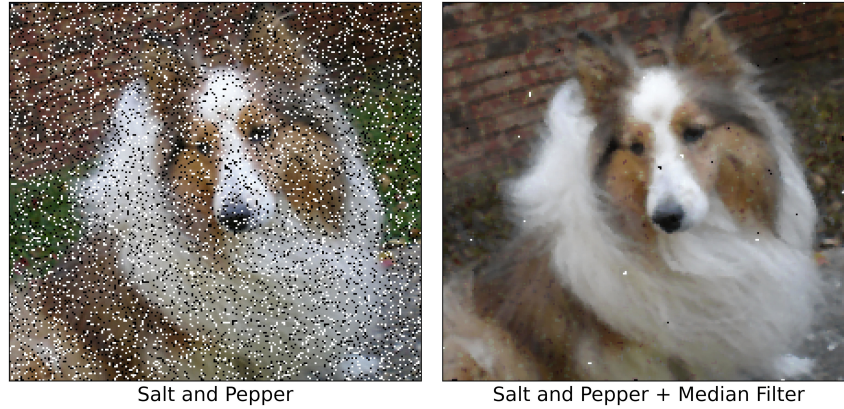
Figure 6.2.1: To the left: An image from the ImageNet dataset distorted with salt and pepper noise. To the right: The same image after a median filter has been applied. The image to the right is visually less distorted to the human eye but slightly blurred.
