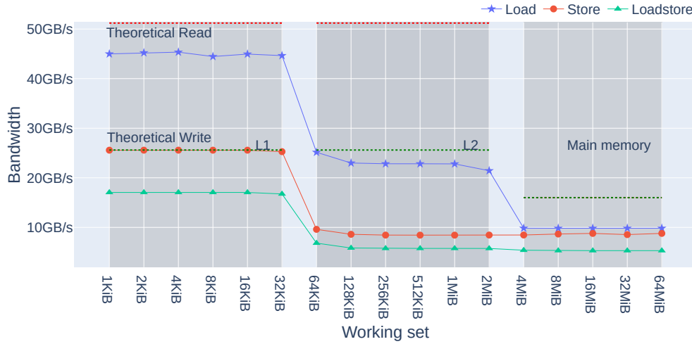
Figure 6.1: Memory bandwidth when running the streaming microbenchmark for different sizes of working sets.
