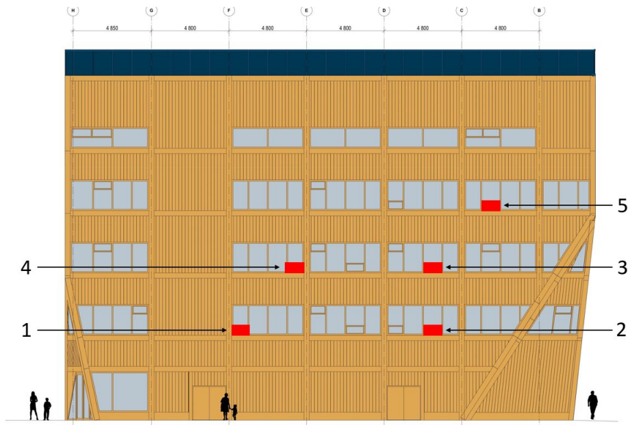
Figure 6.3: Placement of the five sensors on the north facade and their respective sensor number.
