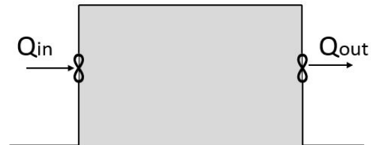
Figure 3.2: Illustration of balanced mechanical ventilation with one supply fan and one exhaust fan.
