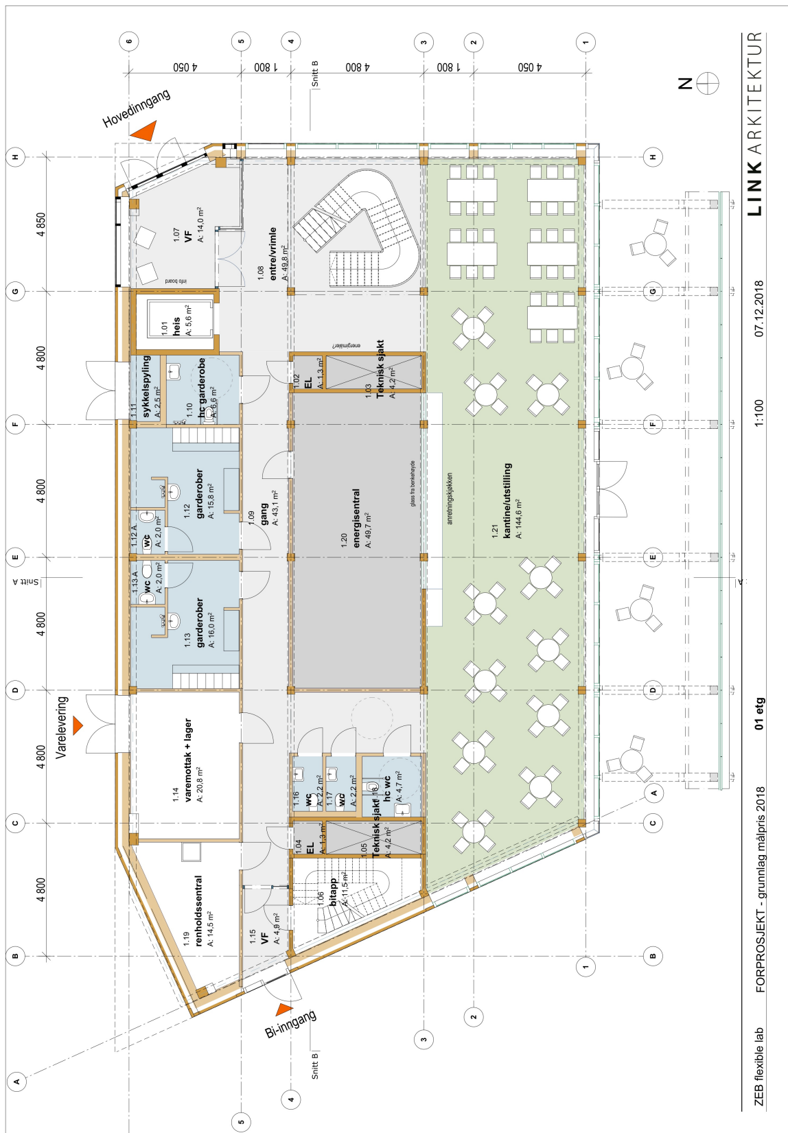
Figure B.1: Floor plan of the first floor of the ZEB Laboratory.
