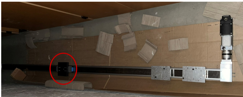
Figure 4.15: A photograph of the traverse used to move the laser probe. The wagon the probe was mounted to is highlighted by the red circle.
