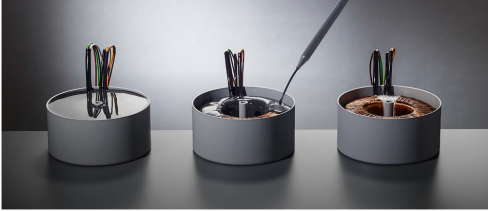
Figure 8: Encapsulation process: Liquid epoxy being applied to copper wires, providing insulation and protection [21]
