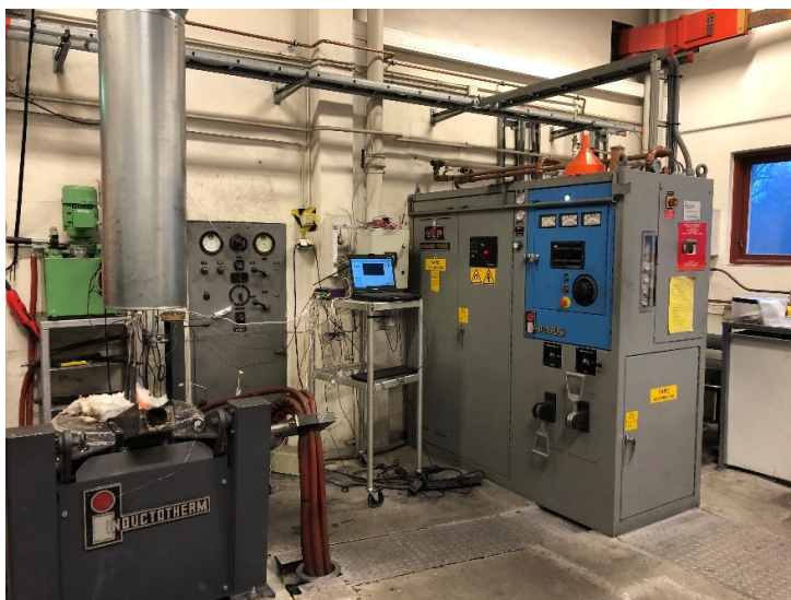
Figure 24. Picture of induction furnace used throughout this work taken by the author.
