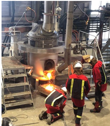
Figure 107. Furnace tapping during pilot scale furnace operations (Photo: Haley Hoover).
