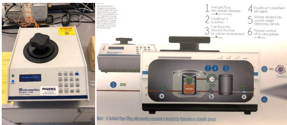
Figure 30. Pycnometer used (left) and schematic of how the instrument works from the manufacturer [75] (right)
