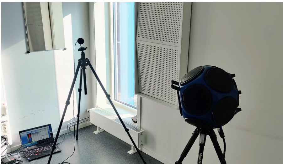
Figure 3.10: Photo of room acoustic measurements in practice room, using pre-calibrated IR setup with omnidirectional microphone and loudspeaker.
