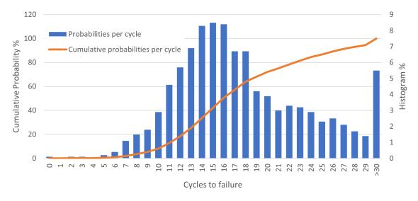
Figure 4.7: Probabilities of failure in the next cycles
