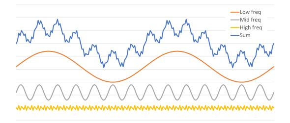
Figure 2.10: Frequency Signals and their composition
