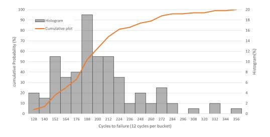
Figure 5.8: Histogram and cumulative plot for total cycles to failure
