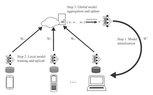
Figure 2.9: Federated learning basic diagram (adapted from Zhang et al. (2021))
