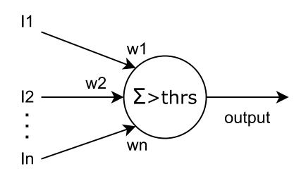
Figure 2.4: Neuron diagram (perceptron). Adapted from Nielsen (2019)
