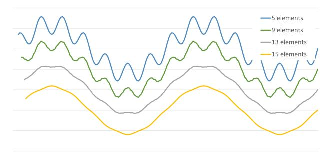
Figure 2.11: Filtering by moving average. 5, 9, 13 and 15 window width
