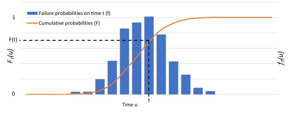
Figure 2.3: Failure Probability and Reliability for observed failure times
