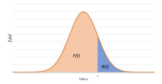
Figure 2.2: Failure Probability and Reliability at time t
