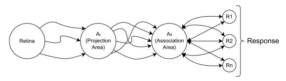
Figure 2.5: Vision Neural Network model. Adapted from Rosenblatt (1958)
