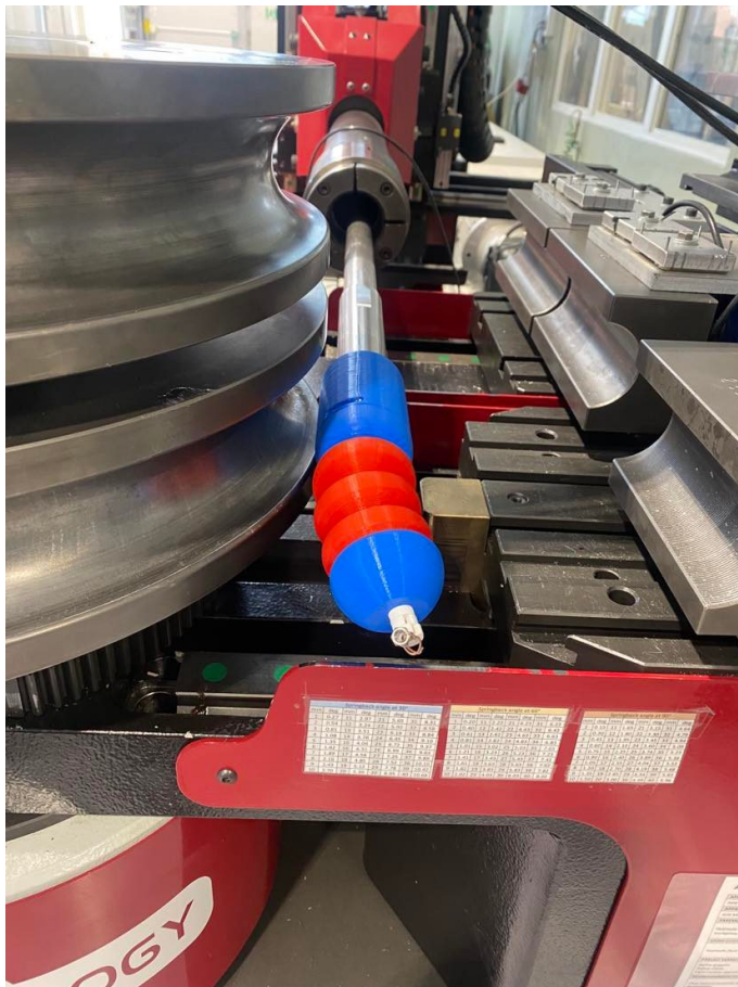
(a) Assembled mandrel in RDB
