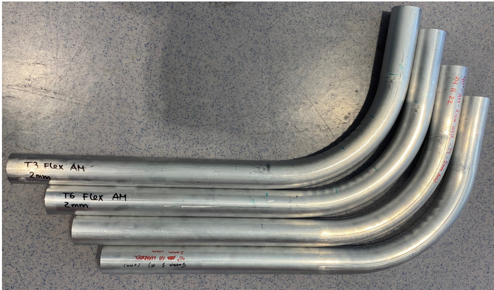
Figure 37: Rigid mandrels on 2mm tube.
