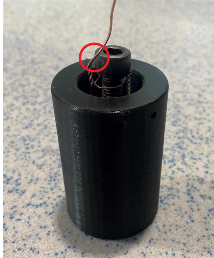
(b) Red ring around wire fracture
