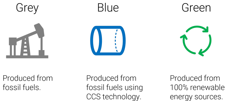
Figure 2.4: Description of alternative fuel production and resulting prefix.
