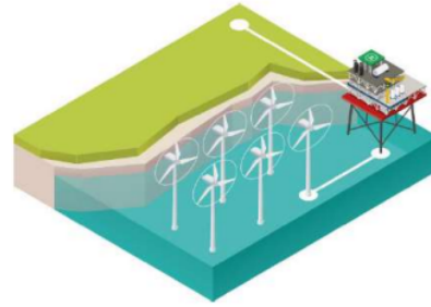
Figure 2.12: Commercial scale offshore hydrogen production coupled with offshore wind farm.[45]
