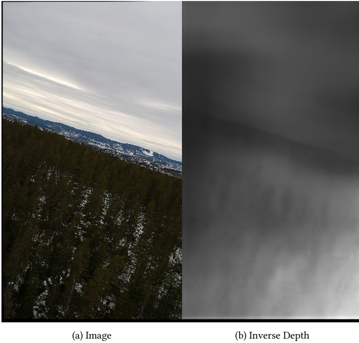
Figure 4.7: Example of poor results during DynaDepth training, indicating inadequate supervision and a challenging estimation problem caused by the lighting and movement.
