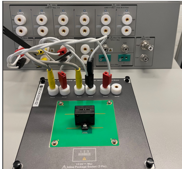
Figure 24: The curve tracer B1505A with the N1265A module from Keysight [91, 92].
