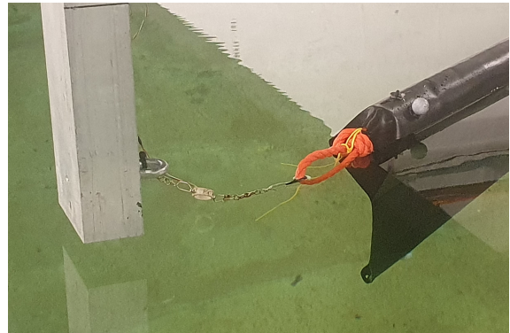
(b) Force transducers connecting the model to the beams
