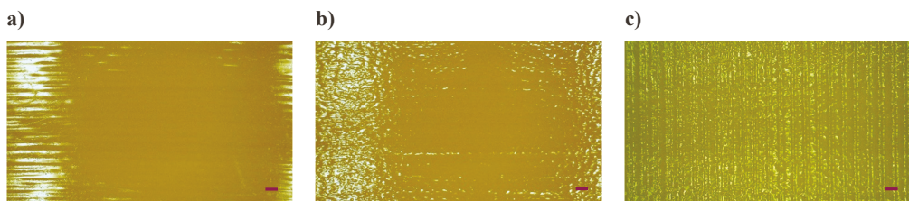
Fig. 20 MJT-printed samples at different wedge angles: a 0°, b 45°, and c 90° (Scale bar represents 1 mm).
