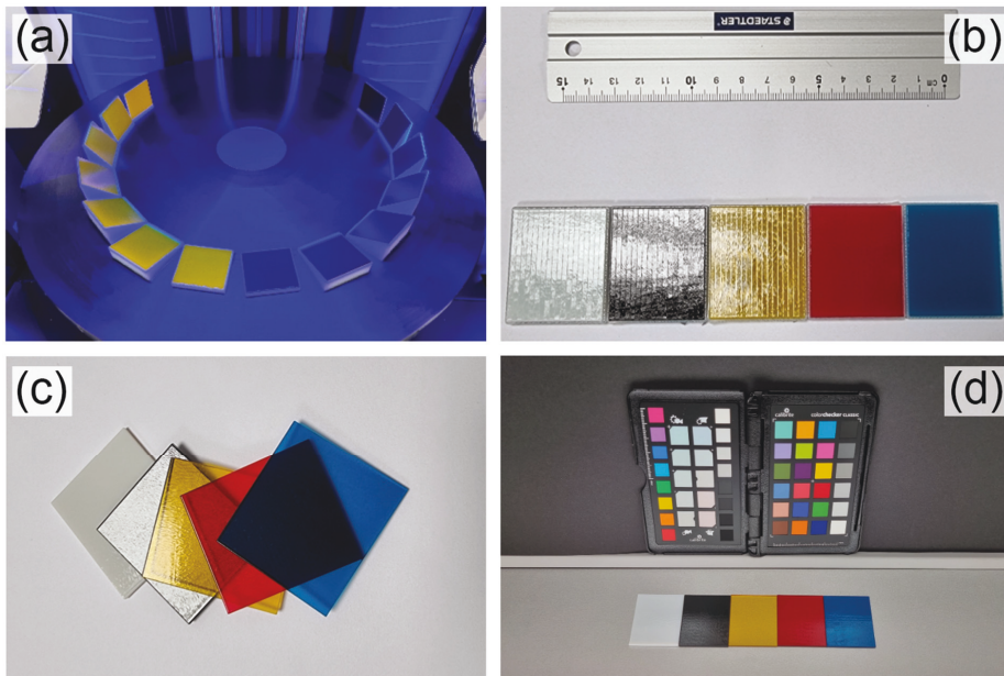
Figure 8. The appearance of objects printed in different conditions using the MJT 3DP technique; Specimens printed at the middle swath and different build orientation ( [0^{\circ}\text{-}90^{\circ}] , 15^{\circ} step) a) on the rotary build platform, b) the appearance and visibility of structured surfaces, c) the translucency in the colored layers, and d) surface appearance under a standard D50 illumination in a light booth.
