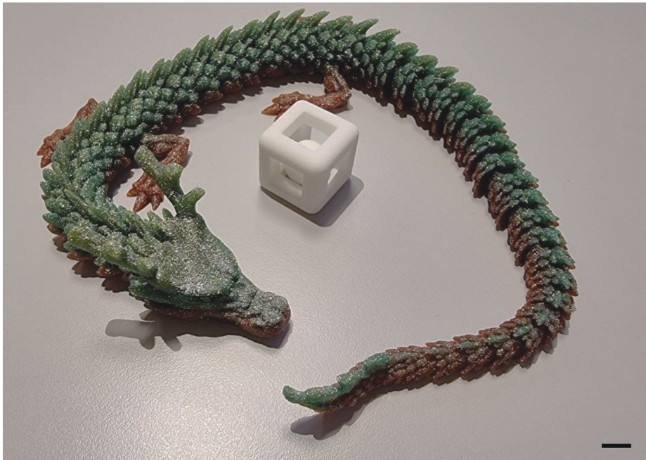
Figure 7. Appearance 3DP in FFF using multicolor PETG filament (the dragon) versus the mono-color-limited SLS printing (the white NTNU 3D logo in the middle); printed at Adlab, the Department of Manufacturing and Civil Engineering – NTNU (Scale bar represents 10 mm).
