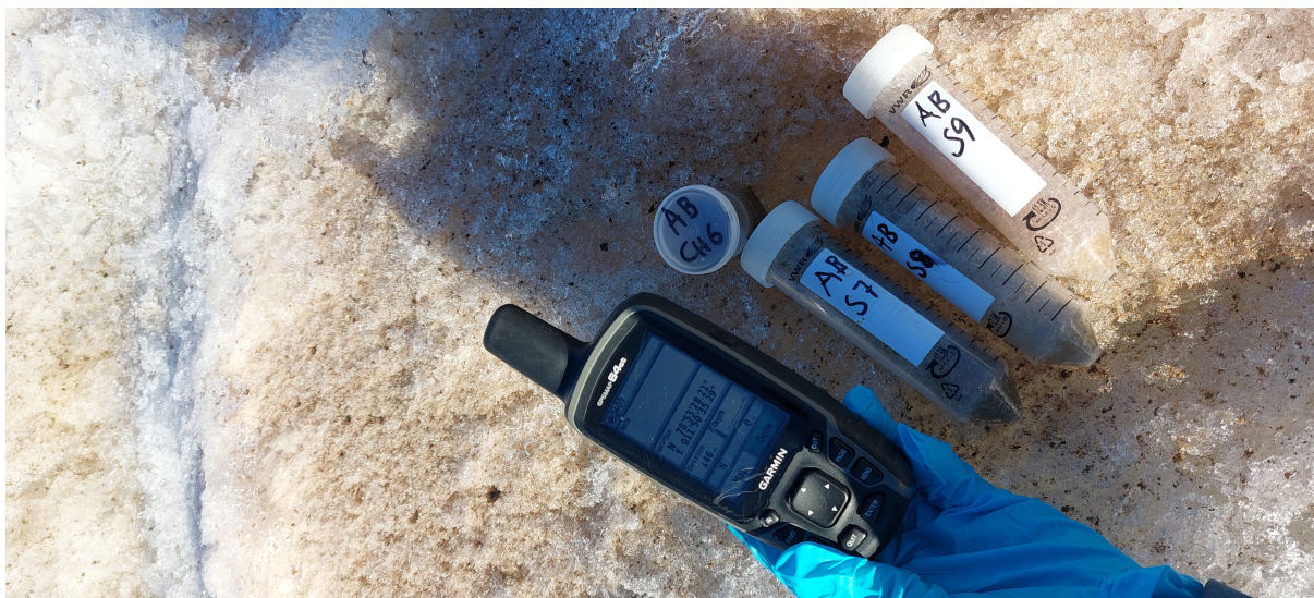
Figure A.1: Snow samples ABS 7, ABS 8, and ABS 9, collected on Austre Brøggerbreen. The colour of the snow is clearly more yellow compared with the other snow samples collected on Austre Brøggerbreen And Vestre Brøggerbreen.
