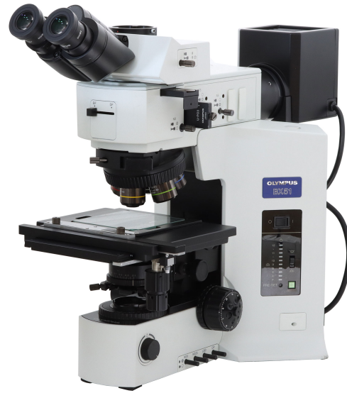
Figure 16: Olympus BX51 Fluorescence Optical Microscope used for scanning of thin sections.
