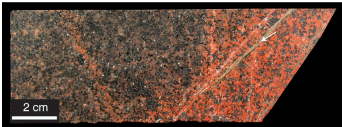
Figure 13: Example of reddening of K-feldspar in vicinity of a fracture. From Plümer and Putnis, 2009.
