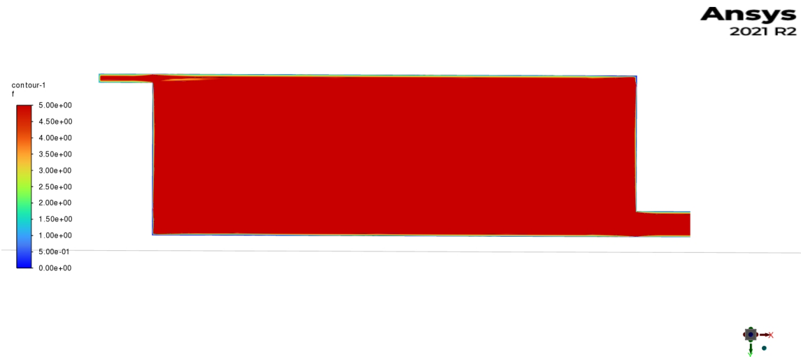
Figure 42: F -value at the xy -midplane of the fully turbulent case gathered from a RANS simulation using the standard k - \epsilon model.
