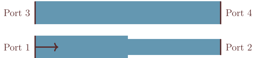
Figure 8.3: Double LPG coupler port configuration during Lumerical simulations. The source port is indicated by the arrow.
