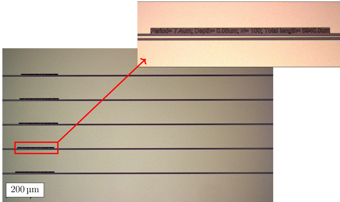
Figure 7.4: Optical micrograph of 5x magnification showing a set of single LPG with grating period \Lambda = 7.4 \mu\text{m} . A summary of important parameters related to each individual waveguide was also patterned as shown by the red arrow.
