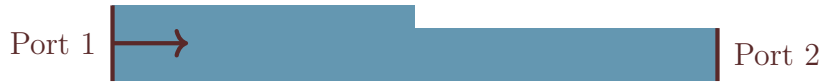
Figure 7.1: Single LPG coupler port configuration during Lumerical simulations. The source port is indicated by the arrow.
